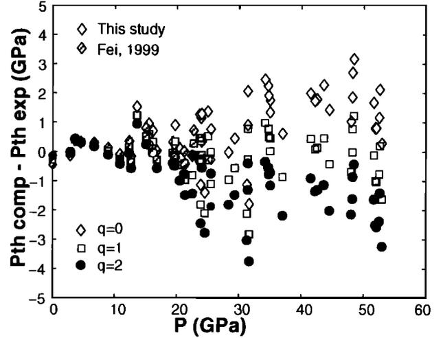
**Figure 4.** Computed difference between  $P_{\text{th comp}} = P(V, T) - P(V, 300 \text{ K})$  estimated from the Debye model, with  $\gamma_0 = 1.45$ ,  $\theta_{D0} = 800 \text{ K}$  (for 3 values of  $q$ ), and  $P_{\text{th exp}} = P(V, T) - P_{\text{BM}}(V, 300)$  for the present measurements and *Fei* [1999] measurements. *Utsumi et al.* [1998] data ( $P < 10$  GPa) are not represented because they do not constrain the  $q$  value.
