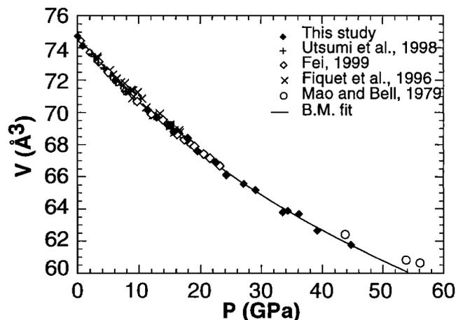
**Figure 2.** Ambient temperature compression curve of MgO, plotted with previous measurements. The solid line represents the Birch-Murnaghan fit of all measurements, except *Mao and Bell* [1979] data, leading to  $K'_0 = 3.94$ , with  $K_0 = 161$  GPa and  $V_0 = 74.71$  Å<sup>3</sup>.
