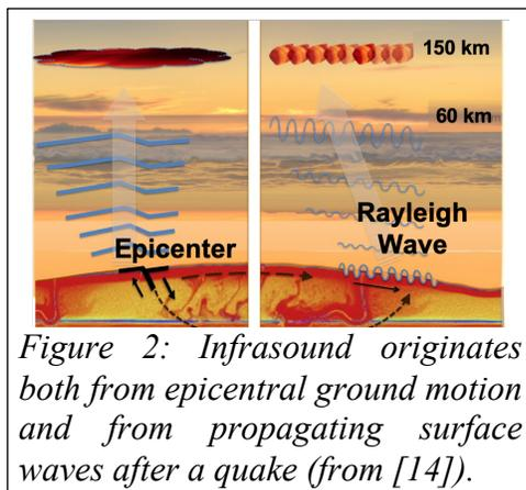
Figure 2: *Infrasound originates both from epicentral ground motion and from propagating surface waves after a quake (from [14]).*
