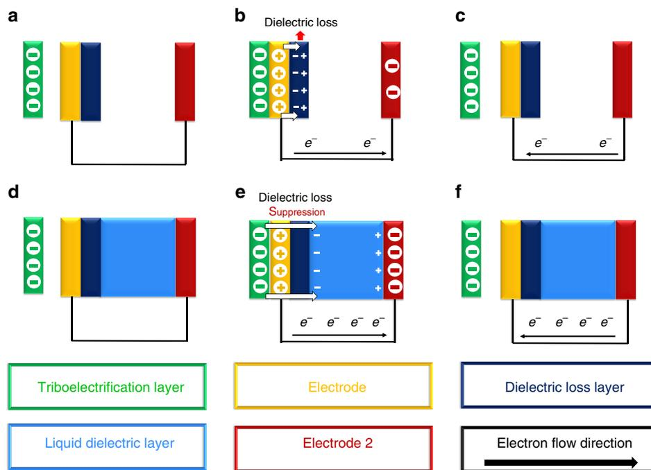
**Fig. 3** Conformation and process of triboelectric generator. **a** Equilibrium state of a TEG without liquid dielectric layer. **b** Contact state without liquid dielectric layer. **c** separation state without liquid dielectric layer. **d** Equilibrium state of a TEG with liquid dielectric layer. **e** Contact state with liquid dielectric layer; and **f** separation state with liquid dielectric layer
