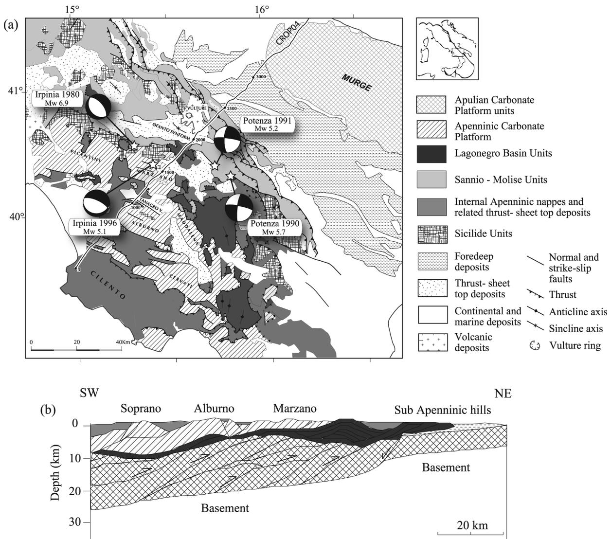
**Figure 1.** (a) Geological map of the Campania–Lucania region (modified from Patacca & Scandone 2007) with locations and focal mechanisms of main large instrumental earthquakes. (b) Schematic cross-section passing through the CROP04 seismic line (modified from Scrocca *et al.* 2005).
