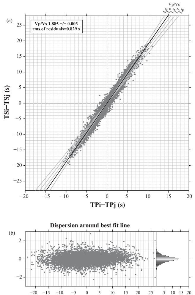
**Figure 3.** (a) ‘Modified Wadati diagram’ showing for each event, and for each pair of station ( $i, j$ ), the difference between  $P$ -phase ( $T_{Pi} - T_{Pj}$ ,  $x$ -axis) and  $S$ -phase ( $T_{Si} - T_{Sj}$ ,  $y$ -axis) arrival times. In black is the best-fit line (which provides an estimate of an average  $V_p/V_s$  ratio of  $1.885 \pm 0.003$ ), in grey are the theoretical lines for several values of  $V_p/V_s$  ratio. (b) Dispersion of the points around the best-fit line.
