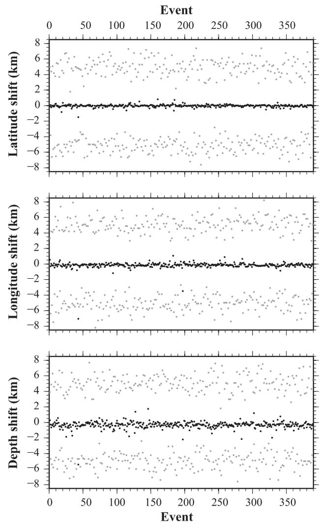
**Figure 5.** Test of VELEST location stability. Initial hypocentre locations, used as reference, are randomly perturbed with a shift of  $\pm 5$  km. Grey dots represent the amount of shift (along latitude, longitude and depth) with respect to the reference locations. The inversion is then repeated, and the retrieved locations shifts are shown as black dots.
