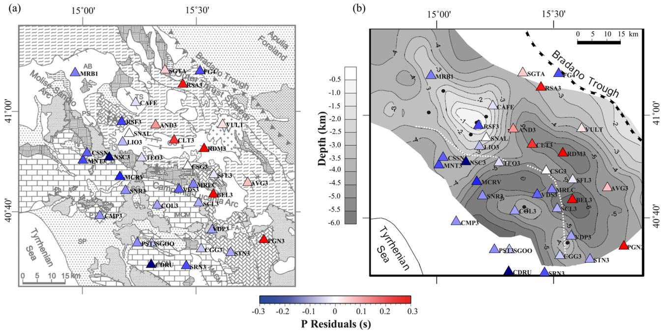
**Figure 9.** Comparison of improved station corrections with (a) a schematic geological map of Campania–Lucania region, and (b) the topography of the top of the Apulian Carbonate Platform (from Improta *et al.* 2003).
