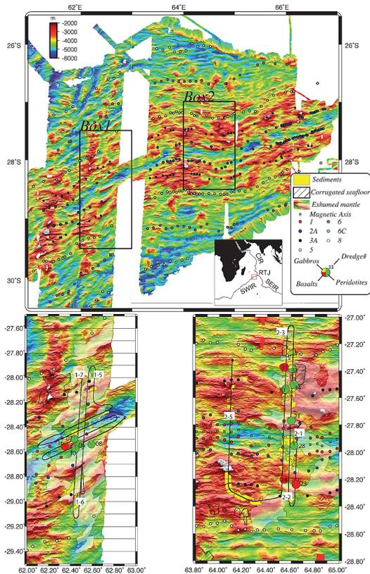
**Fig. 1.** Location of the two survey areas. Magnetic anomaly picks are from Sauter et al. (2008). The nature of the seafloor was deduced either from the side-scan images when available (Sauter et al., 2013) or from the multibeam bathymetric data (Cannat et al., 2006). The dredges numbers and the proportion of rocks by weight shown as pie charts are from Sauter et al. (2013). We have only shown the dredges for which we have measured the magnetic properties (see Table 1 and Figs. 3 and 5)
