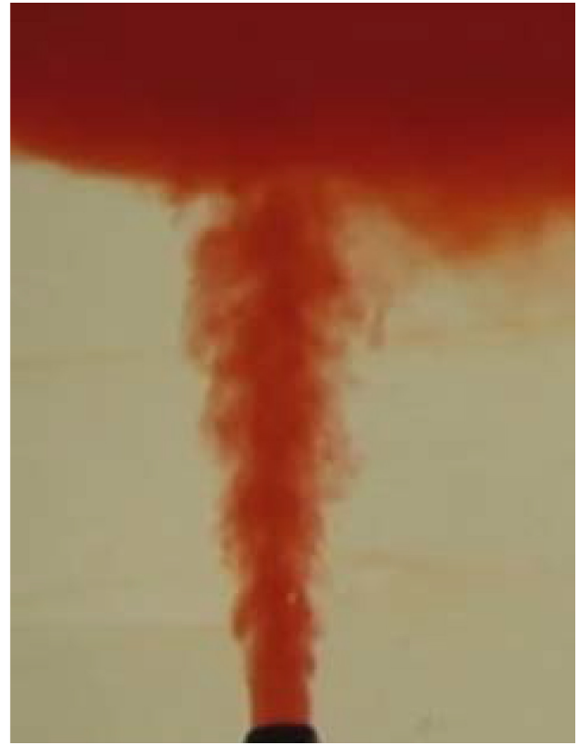
Figure 16. A snapshot from a movie (Carazzo et al., 2014, Supplement Movie S3) recording an experiment simulating a volcanic vent in a stratified water tank.
