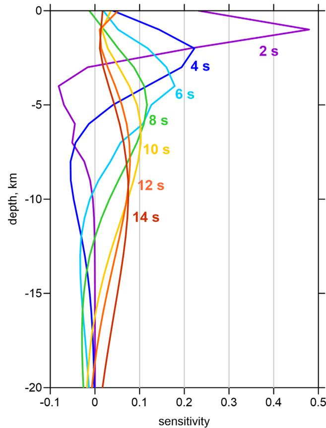
**Figure 8.** Examples of the Rayleigh wave sensitivity kernels for several selected periods indicated with different colors.
