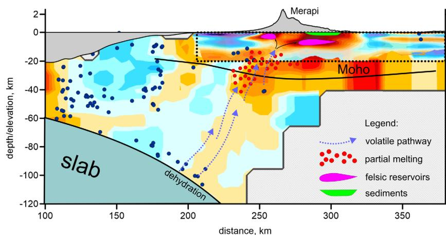
**Figure 14.** Overlapped results of the LET and ANT in the vertical section (same as in Figure 13d) and possible interpretation. Exaggerated topography is shown above the plot. The Moho interface is schematically indicated according to [Wölbern and Rumpker, 2016]. Blue dots are the earthquakes. The gray area depicts the subducting slab. The other symbols are explained in the legend.
