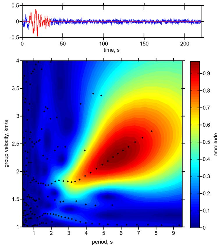
**Figure 3.** Example of the dispersion curve picking at stations AK8 and BJ2 located at the distance of 35.7 km. (top) The Green function for the vertical component seismogram. Red highlights the part, which is processed by the time-frequency analysis. (bottom) The Green function energy depending on the period. Dots indicate all possible dispersion curves.
