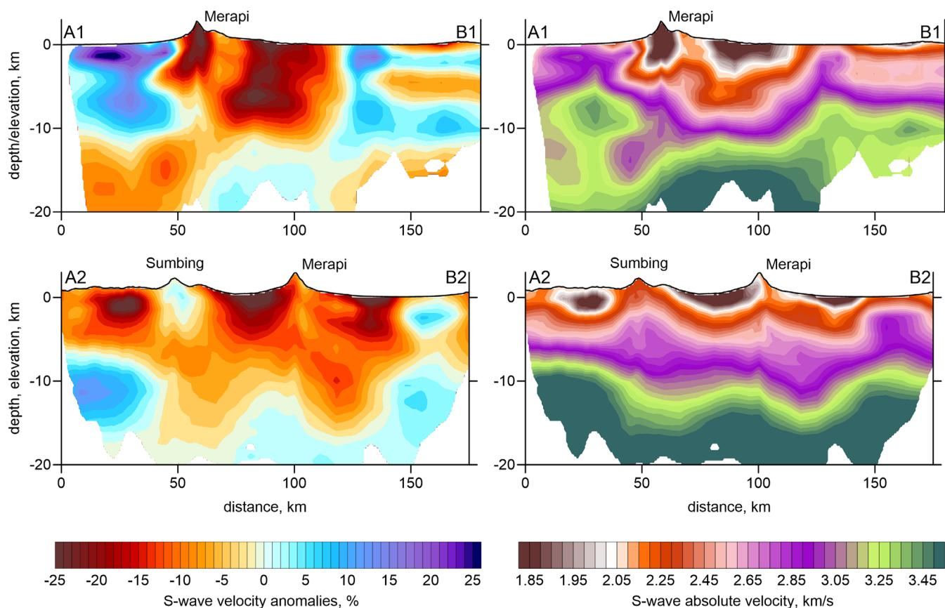
**Figure 12.** Resulting S-wave model in two vertical sections with the locations indicated in Figure 11. Left column present the anomalies, and the right column shows the absolute velocity distributions. The vertical scale is three time exaggerated. The exaggerated topography along the profiles is presented above each plot.
