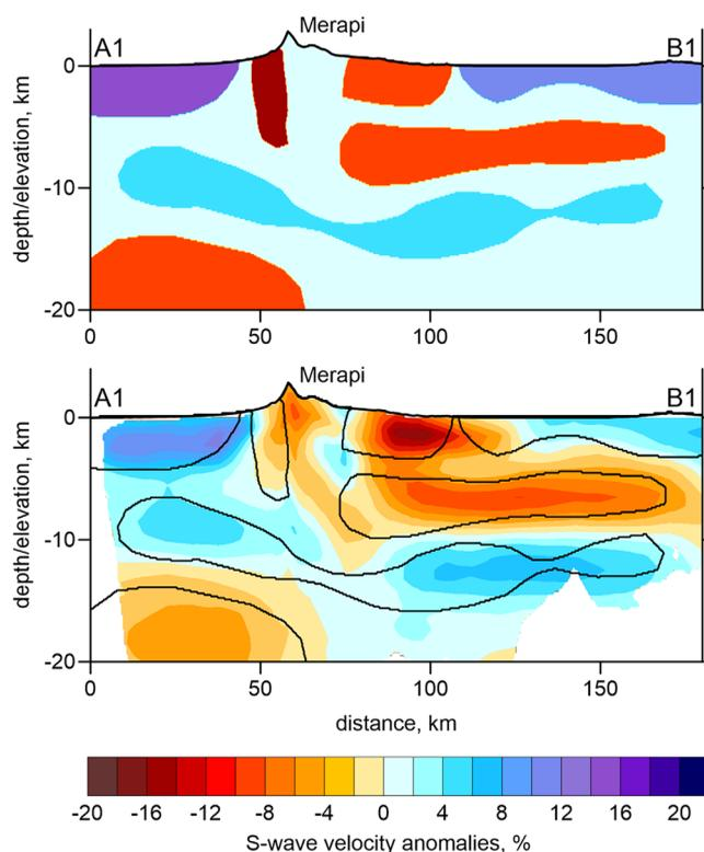
**Figure 10.** Synthetic test with free-shaped anomalies defined in vertical section A1-B1 (See the location in Figure 11). (top) The original synthetic anomalies; (bottom) the recovering result. Think contours highlight the shapes of the original anomalies. The topography along the section is given for the reference.
