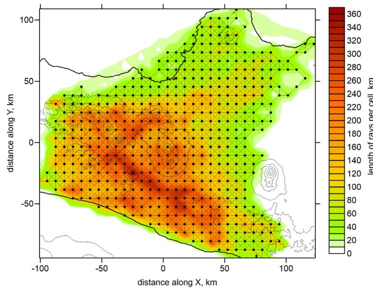
**Figure 6.** Example of ray density and grid nodes of the parameterization grid. Grey lines indicate the links between nodes used for flattening the model during the inversion. Topography is shown by contour lines.
