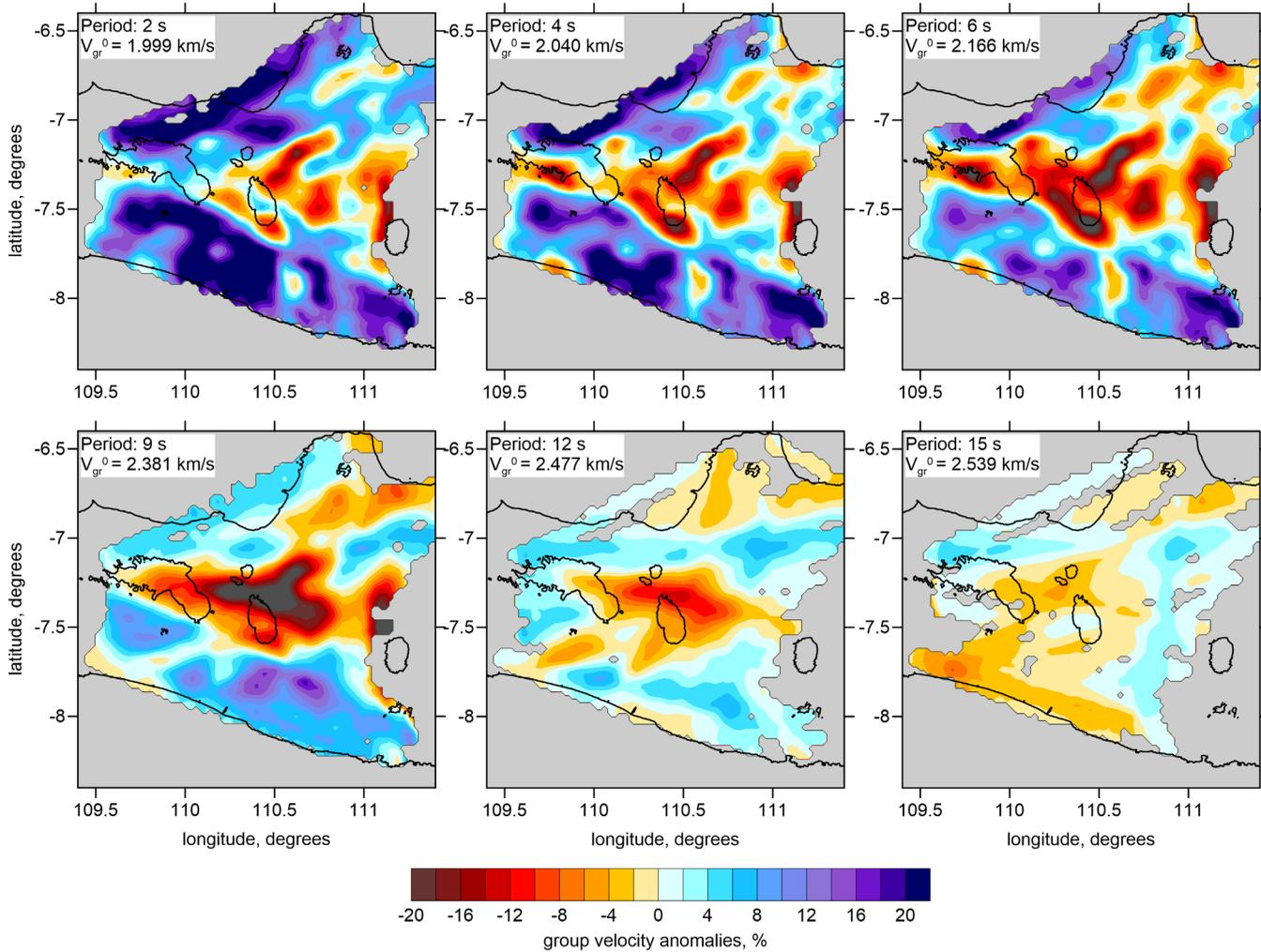
**Figure 7.** Examples of the two-dimensional maps of group velocities deviations for different periods indicated in the top-left corners of each plots. An average group velocity for each period used as reference values are indicated.
