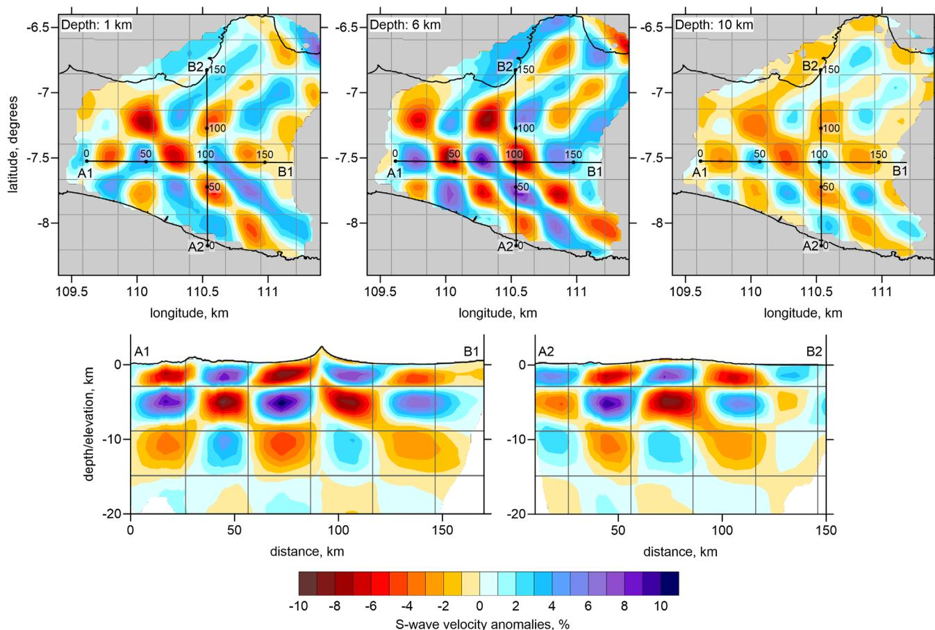
**Figure 9.** Checkerboard test. Upper row shows the recovering result in three horizontal sections. Lower row present the recovering result in two vertical sections with the locations shown in the upper maps. In both cases of horizontal and vertical sections, the gray lines indicate the locations of the true synthetic anomalies.
