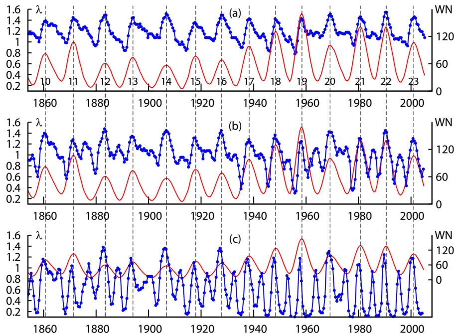
**Figure 1.** The irregularity index  $\lambda$  (blue) computed in a 4-year sliding window for the ISSN averaged over 162 (top panel), 324 (middle panel), and 648 (bottom panel) days; embedding dimension  $m = 1$ . The Wolf numbers averaged first over  $N = 162$ , 324, and 648 days, and then over 4 years are shown in red, together with solar cycle number. Dashed black vertical lines are located at the maxima of ISSN.
