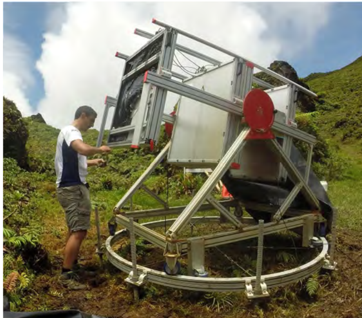
Figure 1.2: View of a field telescope in maintenance on La Soufrière at the Rocher Fendu location. The instrument counts 3 detection matrices (grey frames). A wall of lead bricks with a thickness of 5 cm is placed in front of the central detector. The telescope may easily be rotated to change both its azimuth and its inclination. When in operation, a tarpaulin covers the instruments to protect it against rain. Reprinted from Jourde et al. [2016b].
