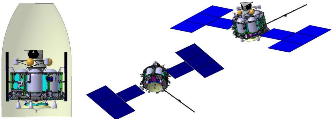
Figure 2: Spacecraft configuration (stacked and deployed)
