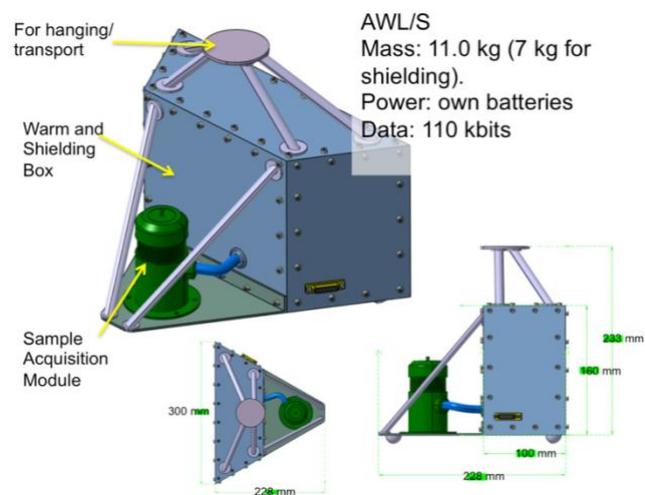
*Figure 4: AWL/S mechanical configuration concept. A support structure allows it to be handled by the lander arm. A box protects the electronics, MAP and MPP. The isolation lid, below SAM, has a lateral movement to be open.*
