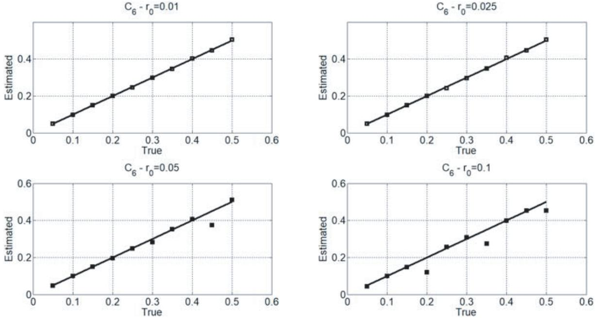
**Figure 11.** Value of thickness of the snow cover estimated from a set of noisy incoherent intensities as a function of the true value for the C6 configurations (bi-exponential autocorrelation function — Anisotropic case).
