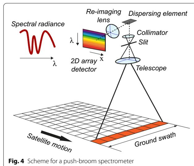
**Fig. 4** Scheme for a push-broom spectrometer
