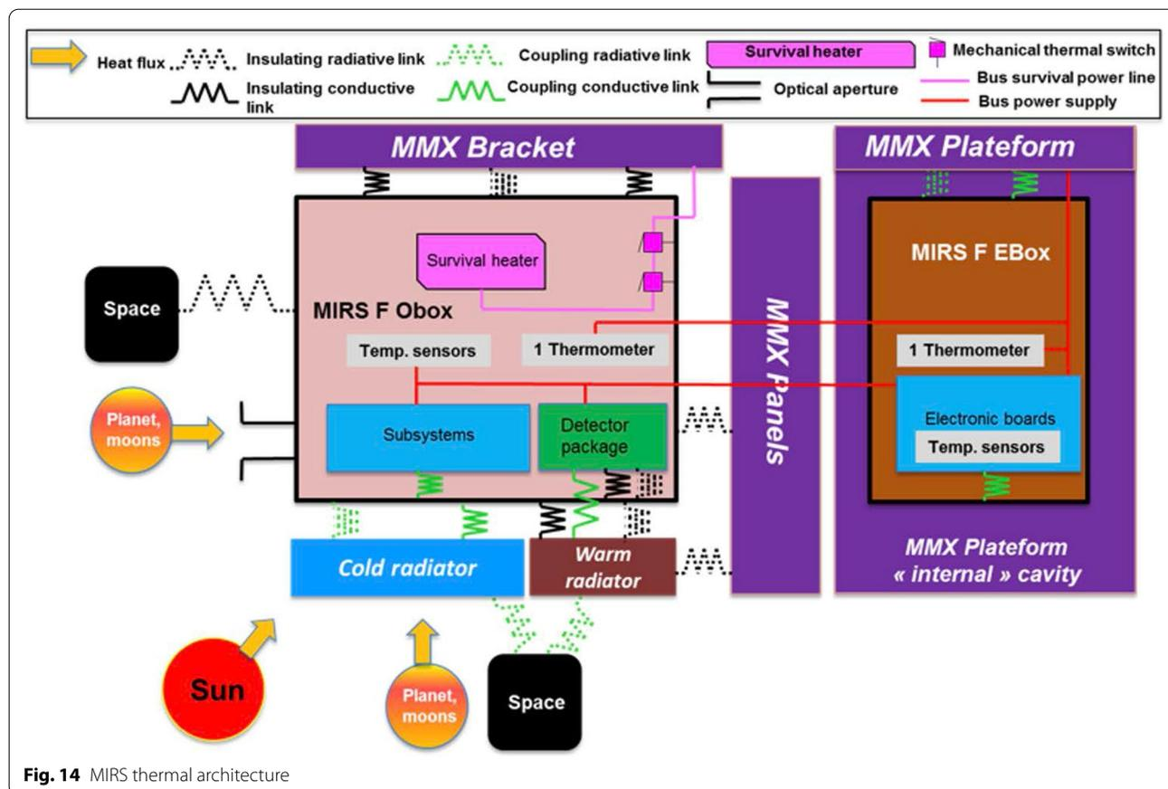
Fig. 14 MIRS thermal architecture
