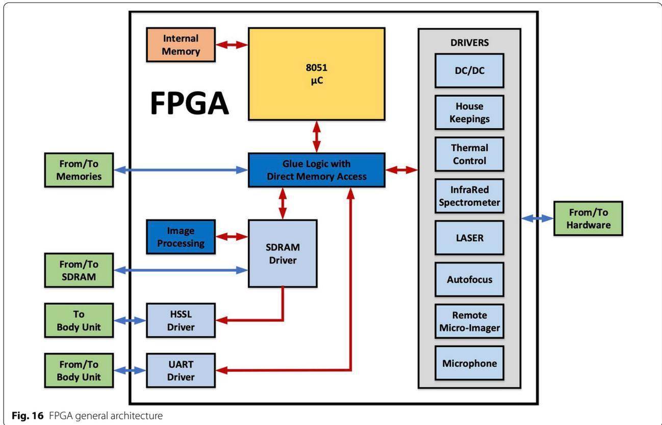
Fig. 16 FPGA general architecture
