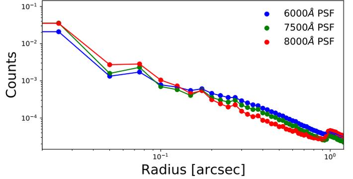
**Fig. 4.** Comparison of the three MUSE AO PSFs we derived using the maoppy code. This is a radial profile taken from the full 2D PSF that the maoppy code provides on the same 0.025'' pixel size as the MUSE data. The variation of the data points are due to the MUSE pixel size in which the PSF was generated.
