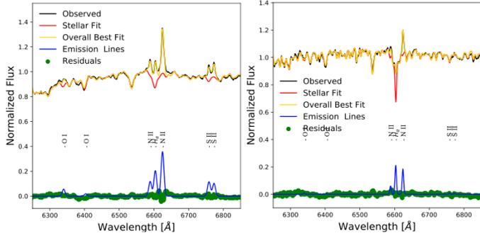
**Fig. 13.** Part of the integrated spectra of Nucleus 1 (*left panel*) and Nucleus 2 (*right panel*), showing a zoomed-in image of the area containing the [NII] $\lambda$ 6583,  $H_{\alpha}$ , and both [SII] lines. The overall best pPXF fit is shown in yellow, the stellar-component is shown in red, and the emission lines are shown in blue.
