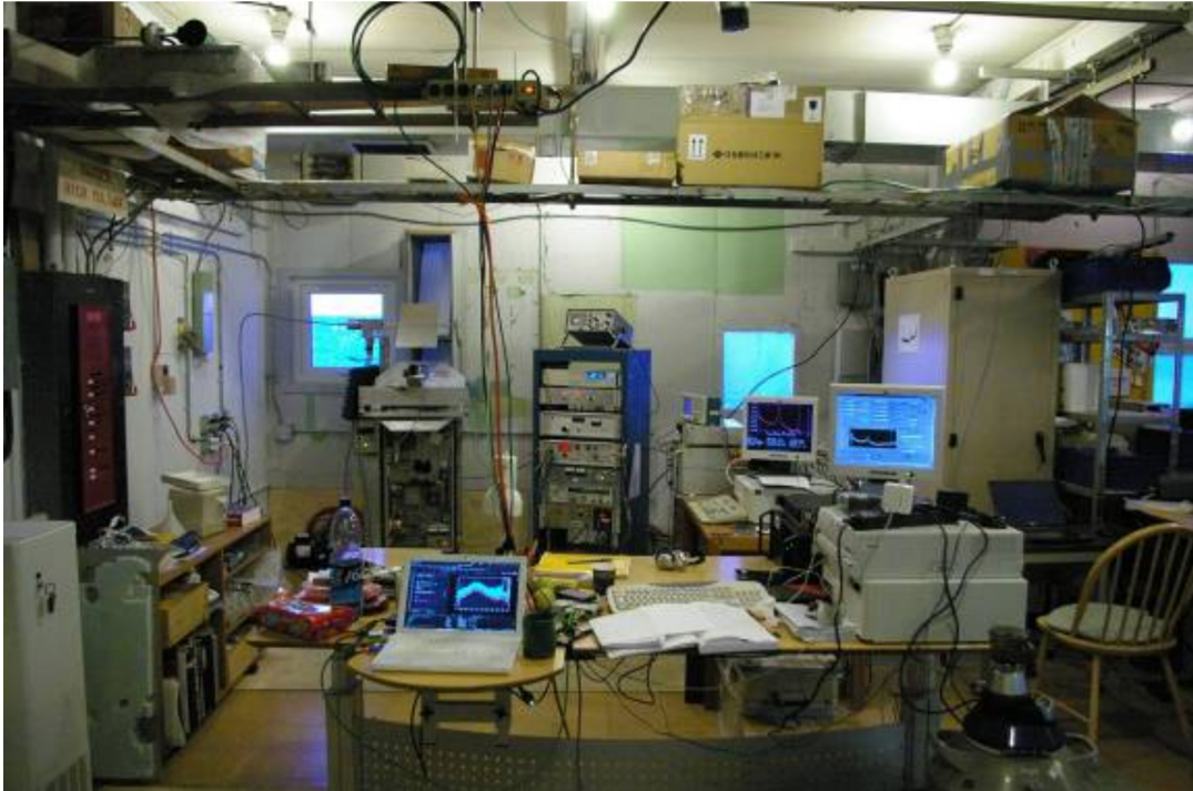
Figure 3. The GBMS installed at Thule, with the receiver facing the mm-wave window.
