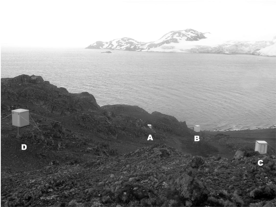
**Fig. 4.** LIV geomagnetic observatory instrument accommodation. The A, B and C huts correspond to the observatory during 1996-2007. They hold the electronics, the absolute instrument and the D/I magnetometer, respectively. The new hut, D, holds the FGE magnetometer deployed during the 2007-2008 summer survey.
