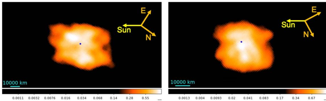
**Figure 5.** Chandra/ACIS-S3 images in the 0.3–0.8 keV energy range for comet 46P. The left panel shows the ACIS-S3 image for epoch 1 (Dec 3); the right panel shows the ACIS-S3 image for epoch 2 (Dec 13) (logarithmic stretch). North, east, and Sun direction are indicated by the arrows. The nominal nucleus position is indicated with a blue circle along with a scale in both images.
