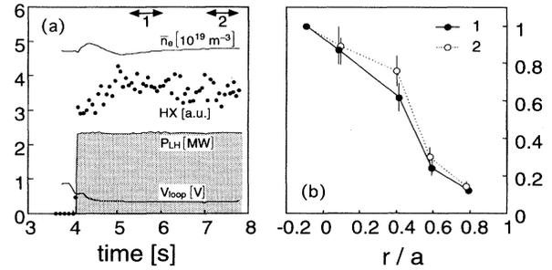
FIG. 1. (a) Time evolution of LH power,  $V_{\text{loop}}$ , line-averaged density, and HXE at  $E = 175$  keV for a central chord. (b) HXE at  $E = 175$  keV (normalized to the maximum value) for the five chords at  $t \approx 5.5$  s (full circles) and  $t \approx 7.5$  s (open circles).
