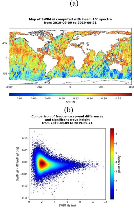
Fig.2 : (a) Map the parameter of spectral width  $\sigma_f$  deduced from the SWIM spectra. (b) histogram of the differences of  $\sigma_f$  values between SWIM and MFWAM as a function of the SWIM significant wave height. The data set is from 9 to 21 September 2019.
