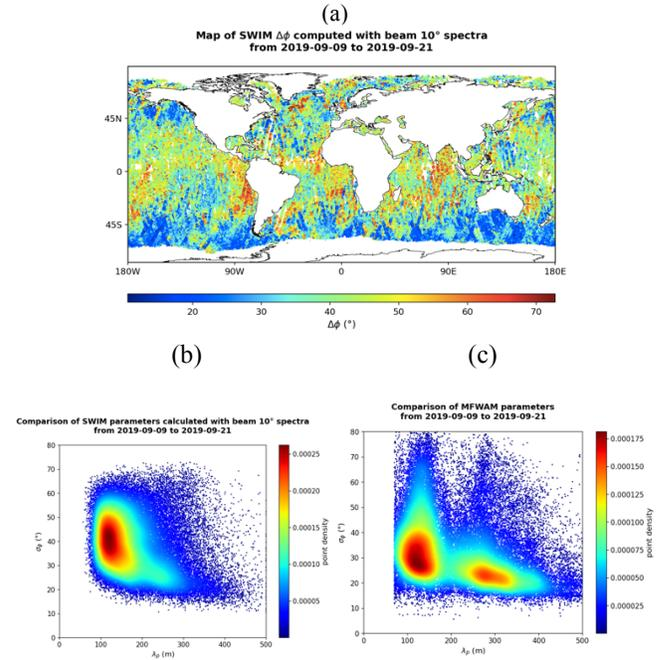
Fig.4 : (a) Same as in Fig2(a) but for the parameter of directional spread  $\sigma_\phi$ , (b-c) : corresponding histograms of the  $Q_p$  values from SWIM (b) or MFWAM (c) as a function of the peak wavelength of SWIM (b) or MFWAM (c).
