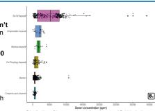
Distribution of boron concentrations in natural fluid inclusions according to the type of mineralization
