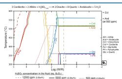
Alteration mineral phase diagram showing the condition of temperature and reaction ratio of a H<sub>2</sub>BO<sub>2</sub>+H<sub>2</sub>O fluid with an assemblage Crd + Alb. Created using CHIM (Reed et al., 2016) and reproducing Weisbrod et al. (1986) experiment
