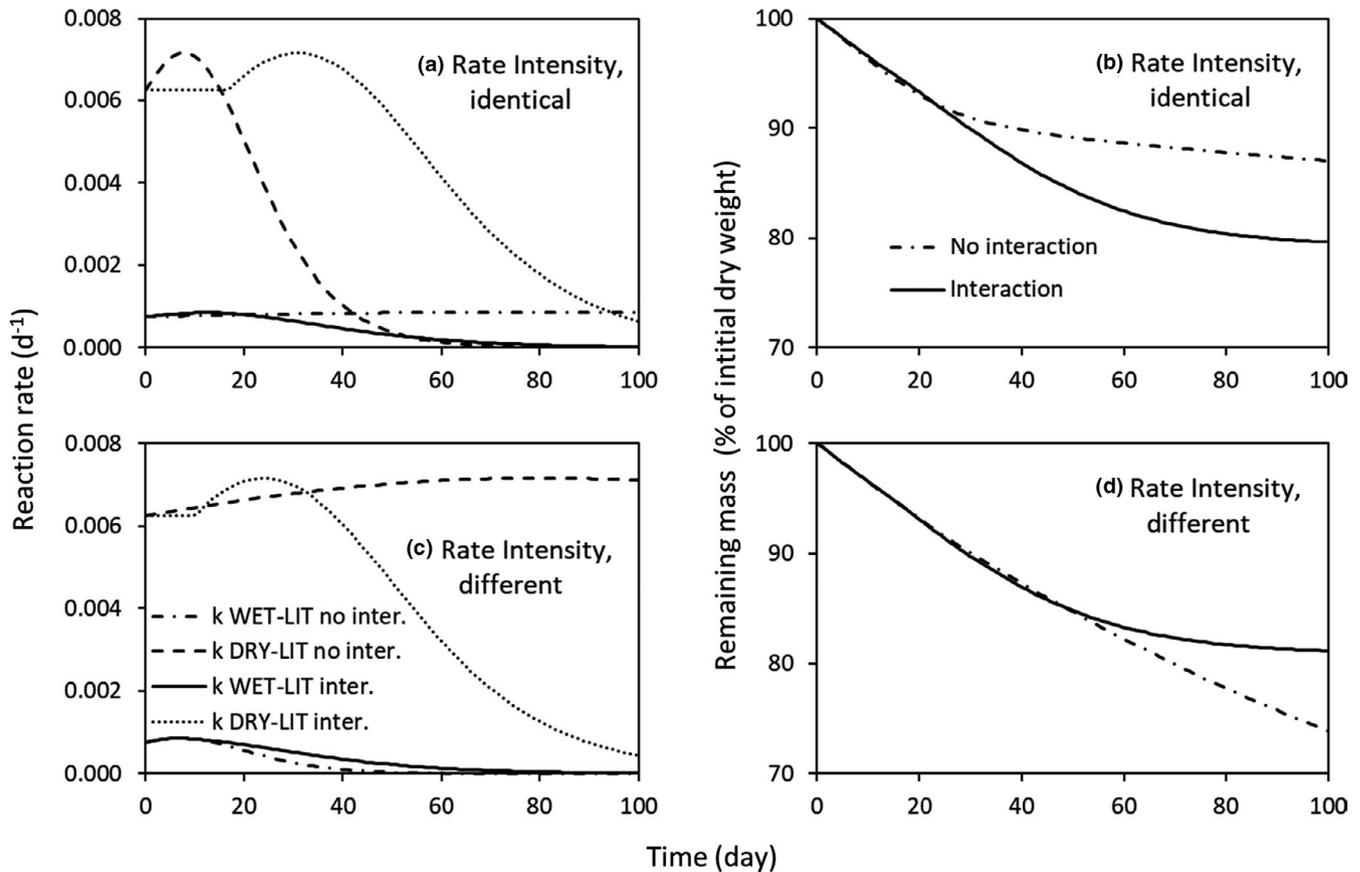
**FIGURE 6** Reaction rates ( $k$ ,  $d^{-1}$ ) and remaining mass (% of initial dry weight) from experiment 2 simulation 1 (a, b, Ex2 Sim1), simulation 2 (Fig. c, d, Ex2 Sim2), and simulation 3 (e, f, Ex2 Sim3). To represent the relationship between the reaction rate and the LWC, Equation 3 from Bunnell et al. (1977) was used in all simulations
