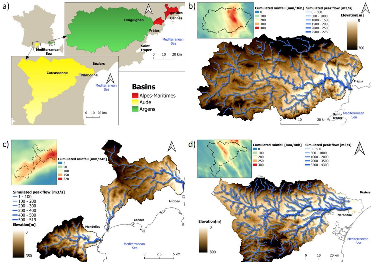
**Figure 2.** Presentation of the three considered areas and flood events, including (a) the location of the watersheds, (b) the Argens 2010 flood, (c) the Alpes-Maritimes 2015 flood, and (d) the Aude 2018 flood. (Map data: IGN; ©Météo France).
