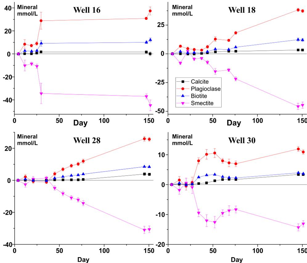
Fig. 14. Cumulative calculated mineral dissolution (+ ve) or precipitation (- ve) from sampled fluids calculated from the difference between each sampling period and the initial sampling period using Eq. (1). Error bars  $1\sigma$ .
