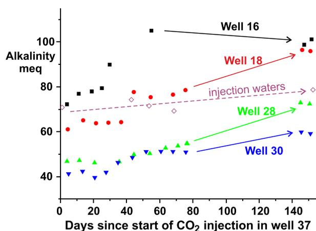
Fig. 8. Variation in alkalinity in produced waters over period after CO<sub>2</sub> injection commenced in well 37. Note that wells to the north already producing significant CO<sub>2</sub> have high initial alkalinities but these continue to rise. Wells 28 and 30 to the south of well 37 have low initial alkalinities which rise progressively during the sampling period. Data averaged over 4 to 8 day periods.
