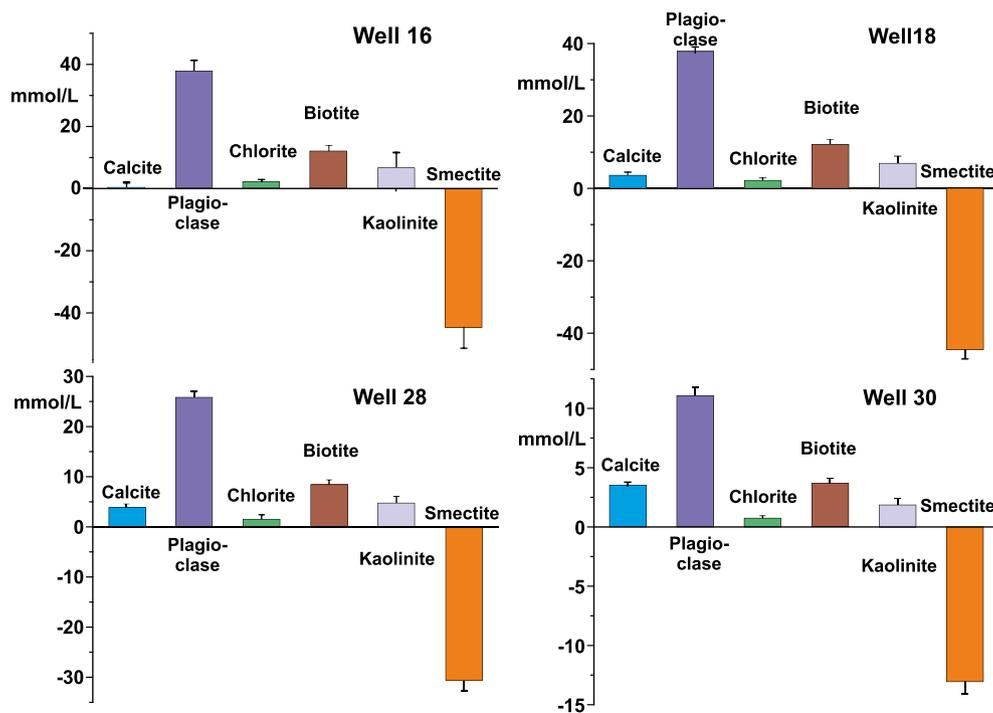
**Fig. 12.** Mineral inputs (negative for precipitation) in mmol/L calculated from difference between initial and final fluid samples (Eq. (1)) for the four wells and solved for the components Si-Al-Mg-Ca-Na-K. Error bars are 1 $\sigma$  calculated from uncertainties in mineral and fluid compositions.
