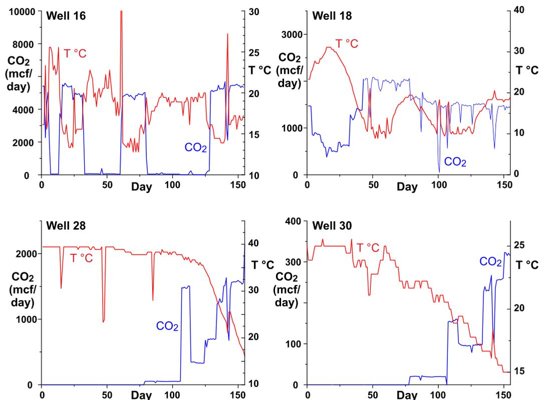
Fig. 6. Recorded CO<sub>2</sub> production (mcf/day) and production temperatures for wells 16, 18, 28 and 30WC2NW05. Drops in temperature reflect cooling from expansion of an increased fraction of the produced CO<sub>2</sub>. Times of near-zero CO<sub>2</sub> production in well 16 reflect well shut-in.
