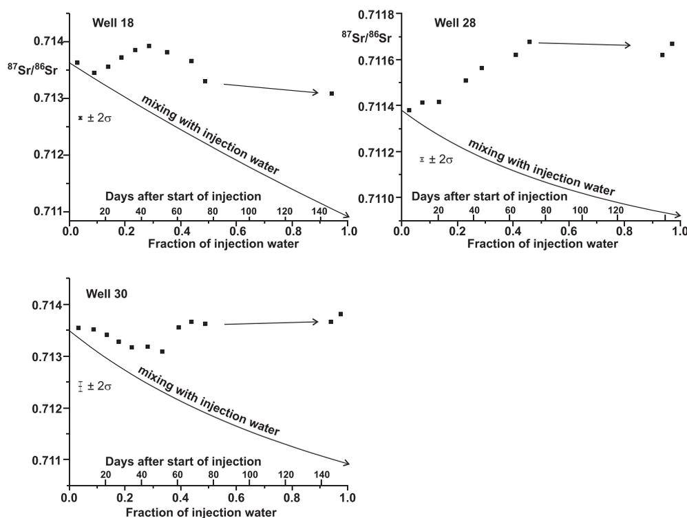
Fig. 11. Calculated mixing curves for  $^{87}\text{Sr}/^{86}\text{Sr}$  ratios between initial fluid samples from wells 18, 28 and 30 as a function of the fraction of initial water added (values below x-axis) compared with time evolution of the sampled fluids (days since injection started given above x-axis).
