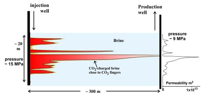
Fig. 5. Diagrammatic 2-dimensional section illustrating how CO<sub>2</sub> will penetrate highest permeability layers. Note expected narrow fringe to CO<sub>2</sub> fingers in which CO<sub>2</sub> diffuses into brine but flow rates in the fringe zone will be proportional to their permeability which is markedly higher than more distal brines.
