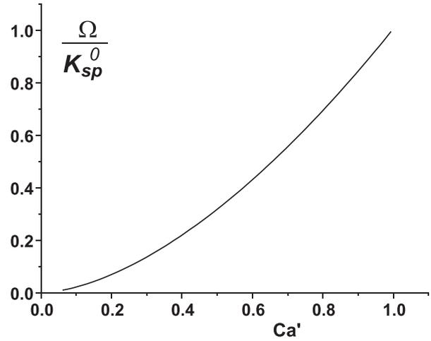
Fig. 16. Variation of calcite saturation state as a function of fluid  $Ca'$  concentration ( $Ca' = Ca/Ca_{eq}$ ) calculated for initial fluid sample SCR-7-28 saturated in CO<sub>2</sub> at 10 MPa and 50 °C.  $Ca_{eq} = 26$  mmol/L.
