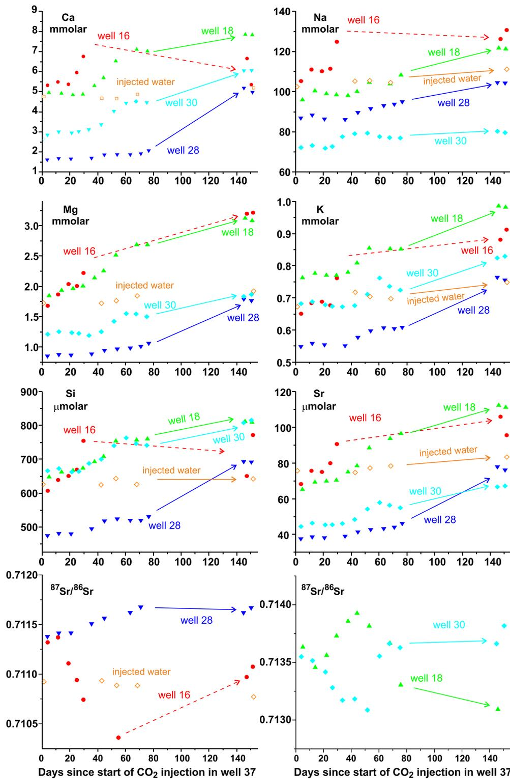
Fig. 9. Variation in Ca, Na, Mg, K, Si, Sr and  $^{87}\text{Sr}/^{86}\text{Sr}$  ratios in produced waters with time after commencement of  $\text{CO}_2$  injection in well 37. Data averaged over 4 to 8 day periods. Open symbols are of injection waters.
