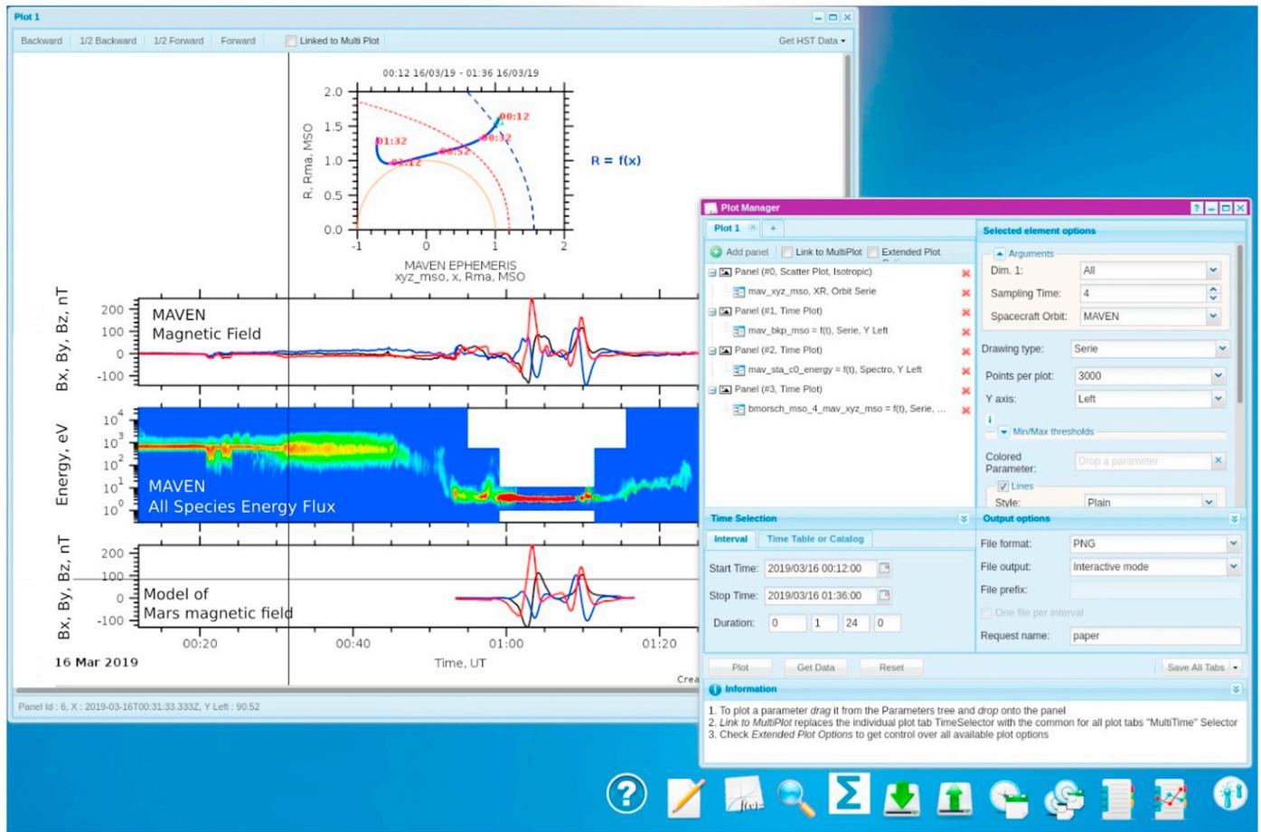
**Fig. 1.** A generic AMDA screen. The plot window shows the MAVEN orbit about Mars, MAVEN magnetic field data, MAVEN Energy-Time spectrogram of the ion energy flux, and the Morschhauser et al. (2014) model of the martian crustal magnetic field calculated along the MAVEN orbit. The right hand side window shows the “plot request” panel set up for this plot. Icons at the bottom right are short cuts to the different analysis activities described in the paper.
