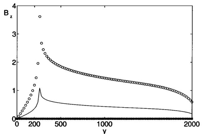
**Figure 4.** The magnetic field  $B_z$  (nT) at 1m above the ground as a function of the distance  $y$  (m) to the symmetry axis. Data are for: c1 (solid line), c2 (\*), c3 (···), c4 (o), c5 (---). c3 and c5 are overprinted by c1.
