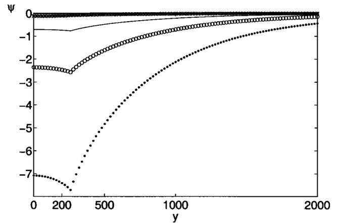
**Figure 3.** The potential field (Volts) on the ground ( $x=0$ ) as a function of the distance  $y$  (m) to the symmetry axis. Data are for: c1 (solid line), c2 (\*), c3 (···), c4 (o), c5 (---). c5 is overprinted by c1.
