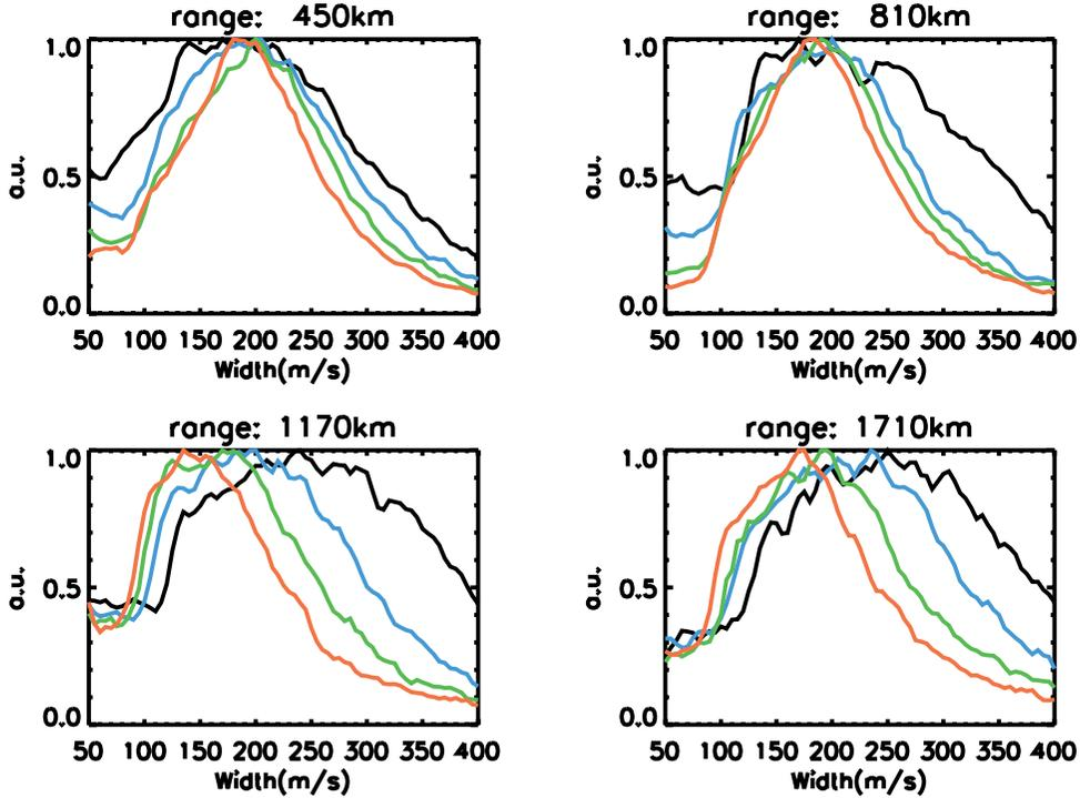
**Figure 6.** Cuts of distribution for 9 MHz (black), 12 MHz (blue), 14 MHz (green) and 16 MHz (red), given for ranges of 450 km (a), 810 km (b), 1170 km (c) and 1710 km (d).
