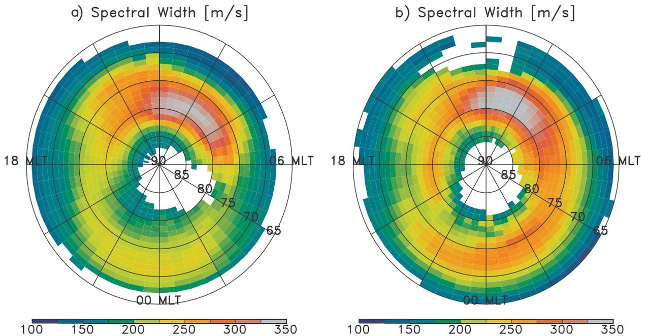
**Figure 9.** Statistical distribution of spectral width values for meridional radars for frequencies greater (a) and lower (b) than 10 MHz in a MLT-MLAT reference frame, with a grid resolution of 30 minutes (MLT) and  $1^\circ$  (MLAT).
