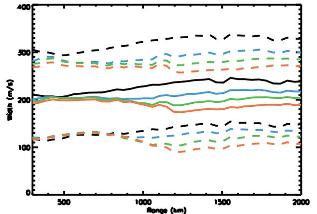
**Figure 7.** Spectral width mean value (solid line) and standard deviation (dashed line) added to and subtracted from the width mean value as a function of range for 9 MHz (black), 12 MHz (blue), 14 MHz (green) and 16 MHz (red).
