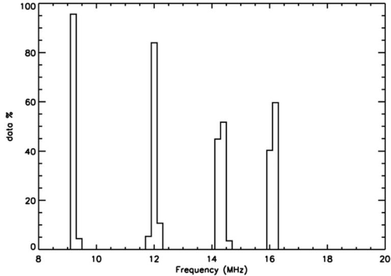
**Figure 2.** Frequency distribution for the database obtained with the multifrequency special mode, showing the echo occurrence at the four selected frequencies, namely 9 MHz (766,739 points), 12 MHz (837,320 points), 14 MHz (784,247 points) and 16 MHz (811,287 points).
