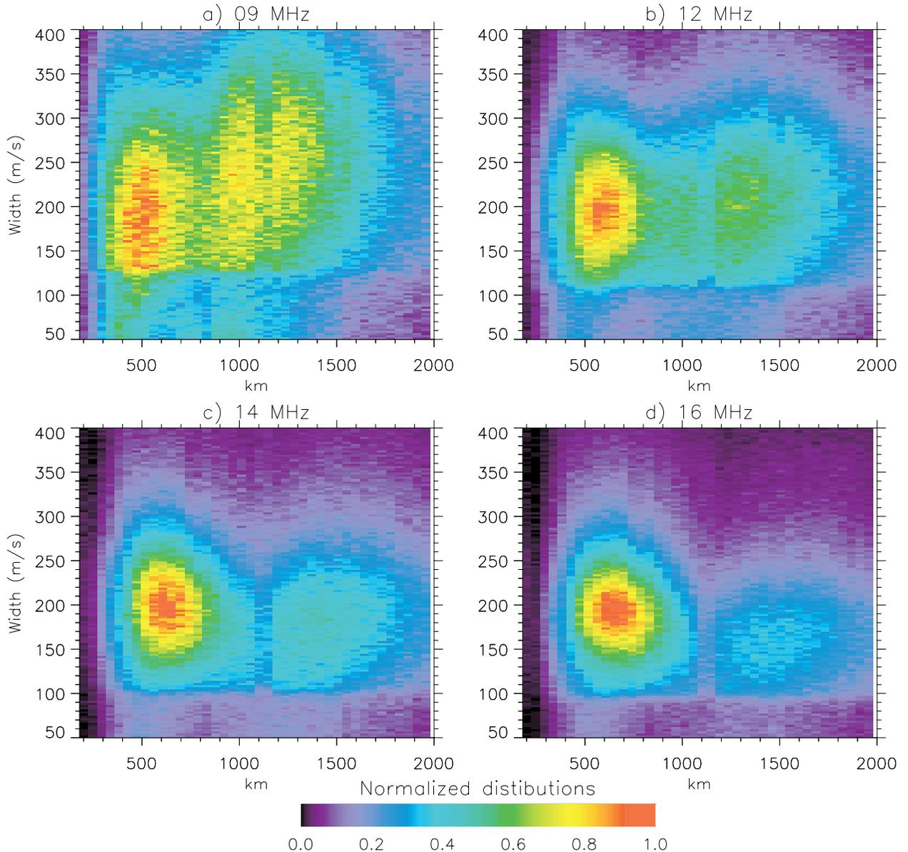
**Figure 4.** Data distribution as a function of spectral width value in  $\text{m.s}^{-1}$  and range for the four frequencies of the special multifrequency mode: (a) 9 MHz, (b) 12 MHz (c) 14 MHz and (d) 16 MHz. Distribution for each frequency is normalized to its maximum value. The grid resolution is 45 km in range and  $5 \text{ m.s}^{-1}$  in width.
