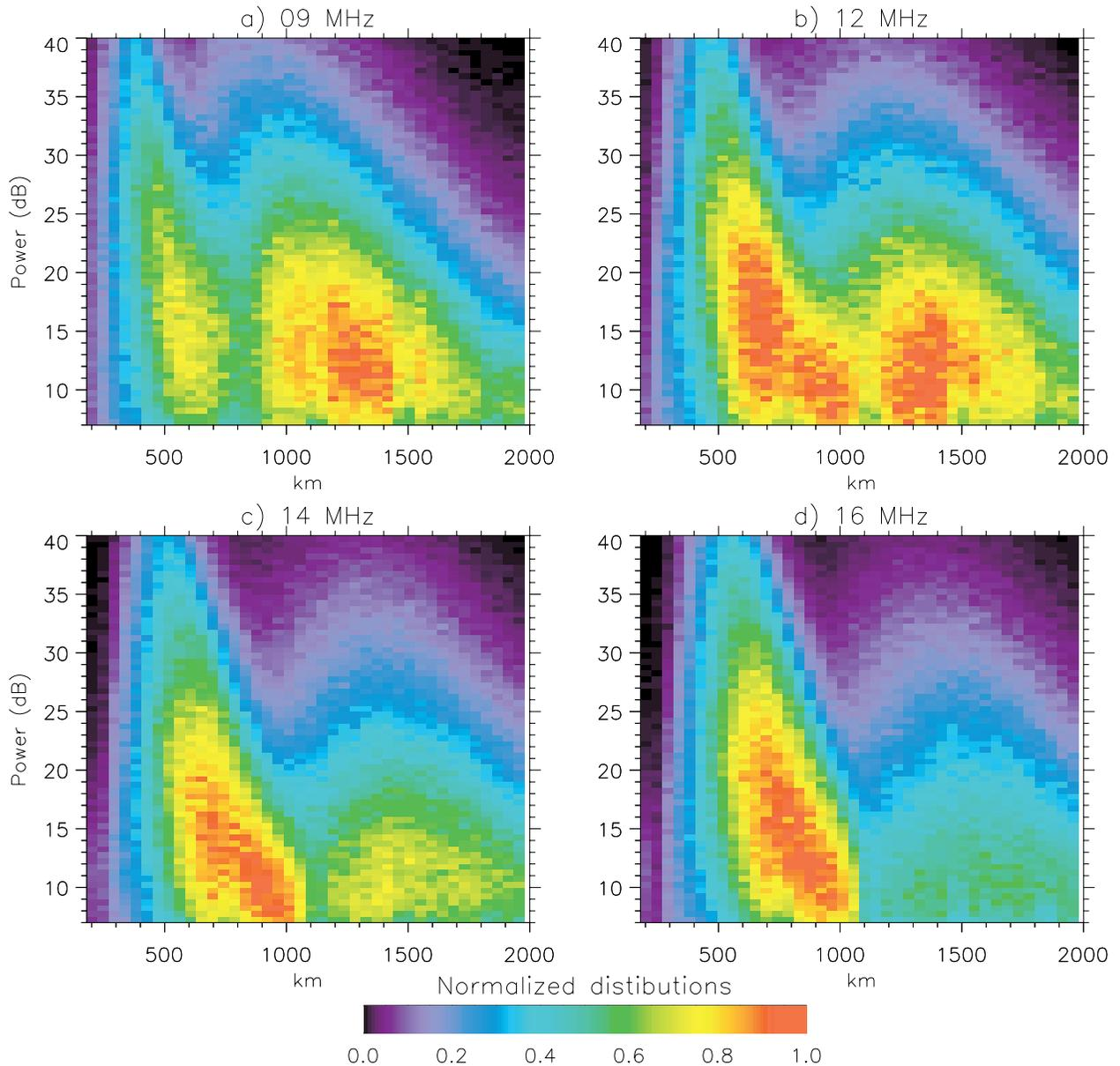
**Figure 3.** Data distribution as a function of power value in dB and range for the four frequencies of the multifrequency special mode: (a) 9 MHz, (b) 12 MHz (c) 14 MHz and (d) 16 MHz. Distribution for each frequency is normalized to its maximum value. The grid resolution is 45 km in range and 1 dB in power.
