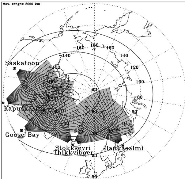
**Figure 1.** Location and fields of view of SuperDARN radars used in this study. The contours in thick line correspond to Invariant Latitude of  $60^\circ$ ,  $70^\circ$  and  $80^\circ$ .
