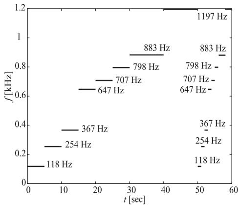
**Figure 1.** Schematic spectrogram (to scale) of the transmission pattern used by the HAARP HF facility to heat the ionosphere. The ELF waves were AM modulated onto a carrier frequency of 3.3 MHz. The transmitted HF wave was in the X mode.
