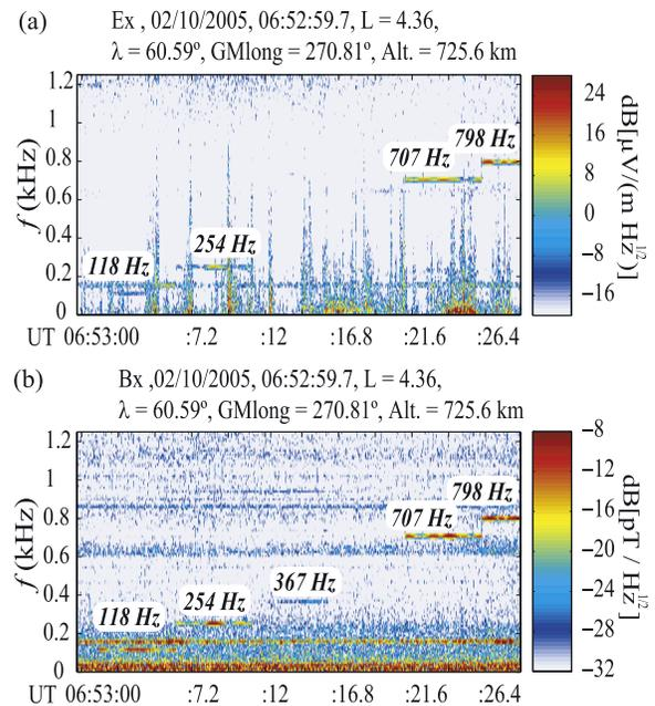
**Figure 3.** Detailed ICE and IMSC spectrograms from the DEMETER satellite pass during February 10, 2005. (a) An overview of the detected HAARP signal in one of the electric field components. The transmitted pattern at frequencies up to 798 Hz is observed. (b) An overview of the detected HAARP signal in one of the magnetic field components. The transmitted pattern at frequencies up to 798 Hz is observed.
