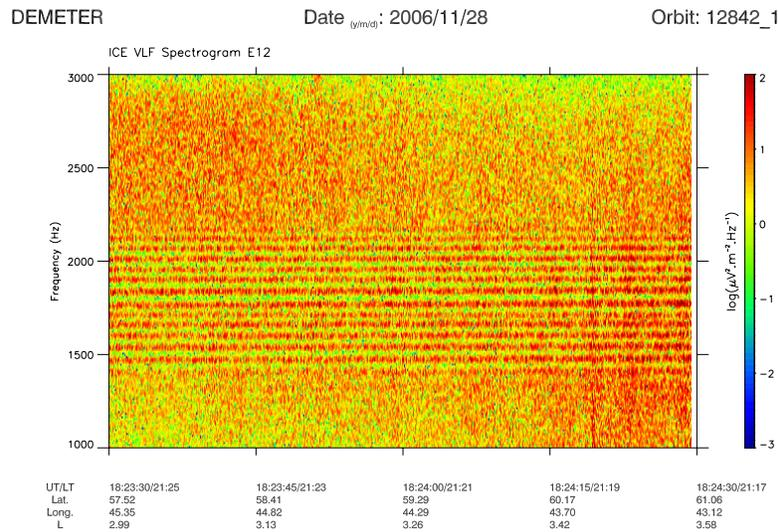
**Figure 3.** Spectrogram of the signal received by the satellite DEMETER between 18.23.30 and 18.24.30 UT at the end of the burst zone shown in Figure 2. The signal intensity is color coded according to the scale on the right. MLR are observed between 1.4 and 2.2 kHz. Orbital parameters are indicated at the bottom: Latitude, longitude and L value. The local time indicates that it is a night time observation.
