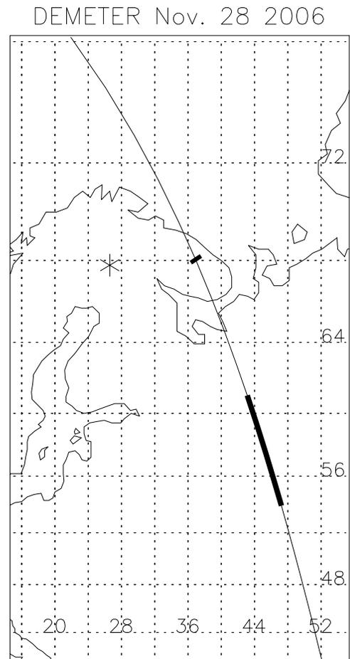
**Figure 2.** Map showing the area where the event has been recorded. The star indicates the position of Kannuslehto (67.74°N, 26.27°E) in Finland. The line represents the projection of the orbit of the satellite DEMETER (12842.1) on November 28, 2006. The thick part shows the location where DEMETER is in burst mode and the tick shows where DEMETER stops to record data.
