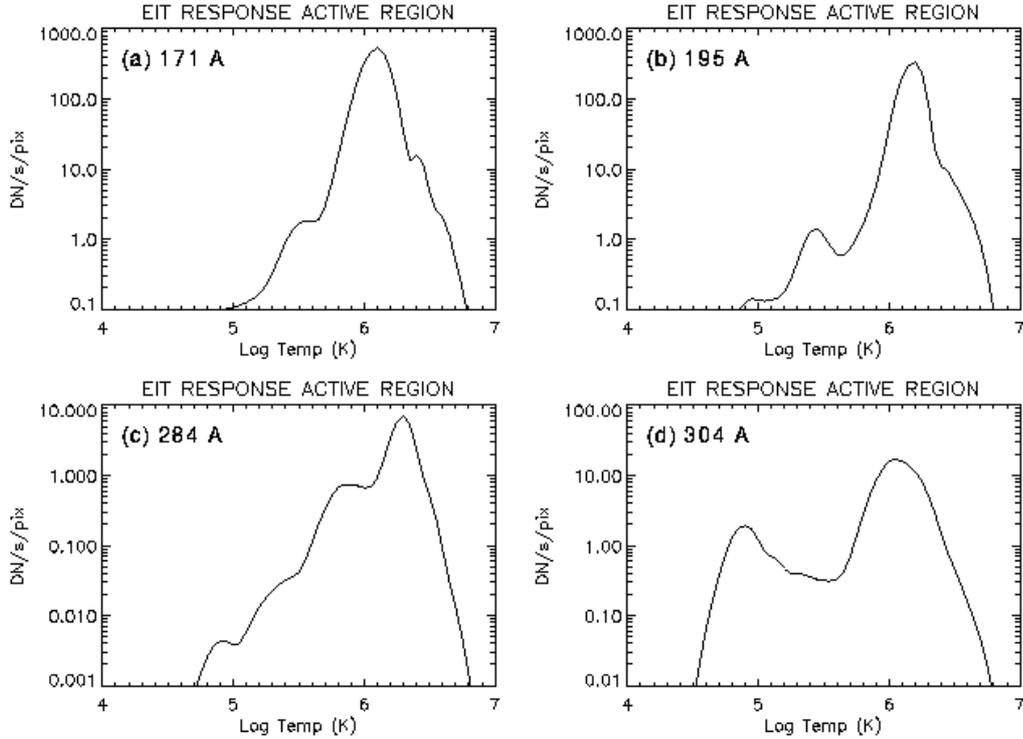
**Fig. 2.** Response of the EIT instrument to the plasma temperature, for an active region computed with an electron density of  $10^9 \text{ cm}^{-3}$  and using the differential emission measure from the CHIANTI model (Delaboudinière et al. 1995).
