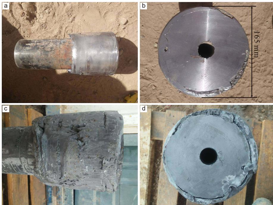
Figure 4. Photos of the lead seal before (a and b) being put into and after (c and d) being pulled out from borehole Shi41H4-3-414. The diameter of the lead seal is 165 mm and the inner diameter of the casing pipe is 172.05 mm. The side face of the lead seal has scratches, but no imprint exists in its bottom surface, which reveals that the coseismic slip at this borehole site is more than the casing pipe diameter of 196.85 mm.
