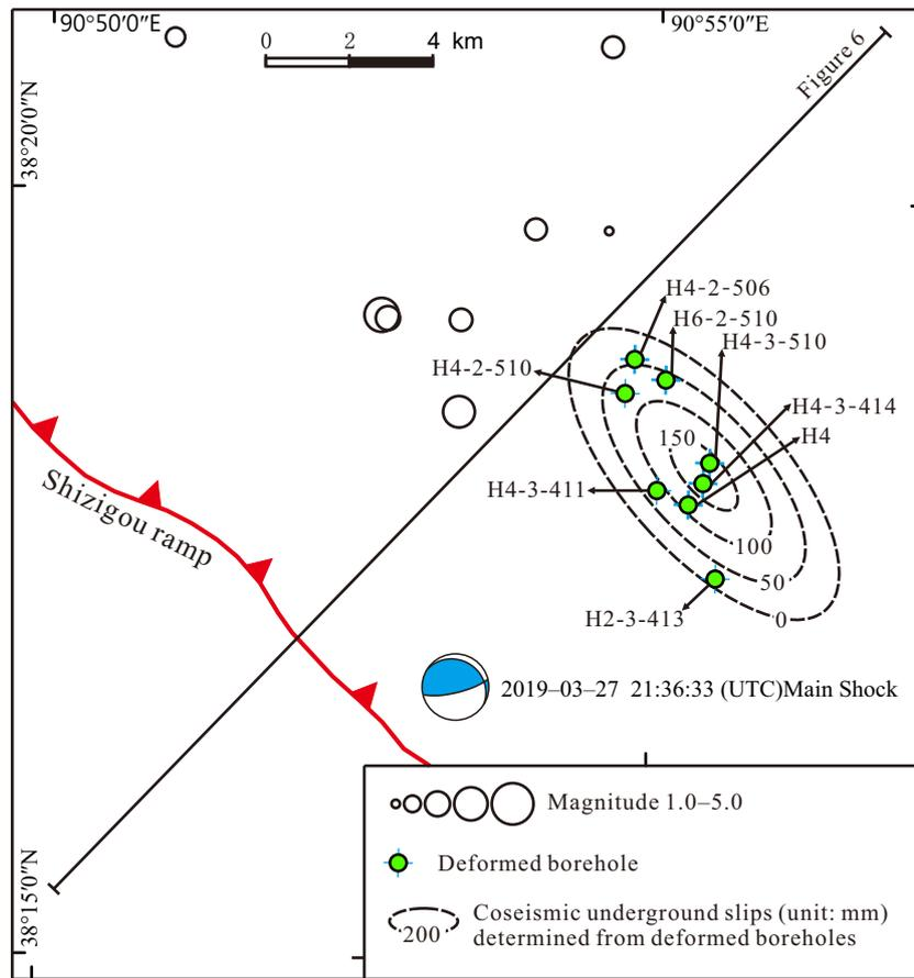
Figure 2. Coseismic slip contour map of the Shizigou (SZG) ramp on the March 28, 2019 Mw 5.04 Mangya earthquake in Yingxiong Ling. Eight damaged boreholes define the coseismic underground rupture area of the event. Epicenters of the main shock and aftershocks are from China Earthquake Data Center (2019).
