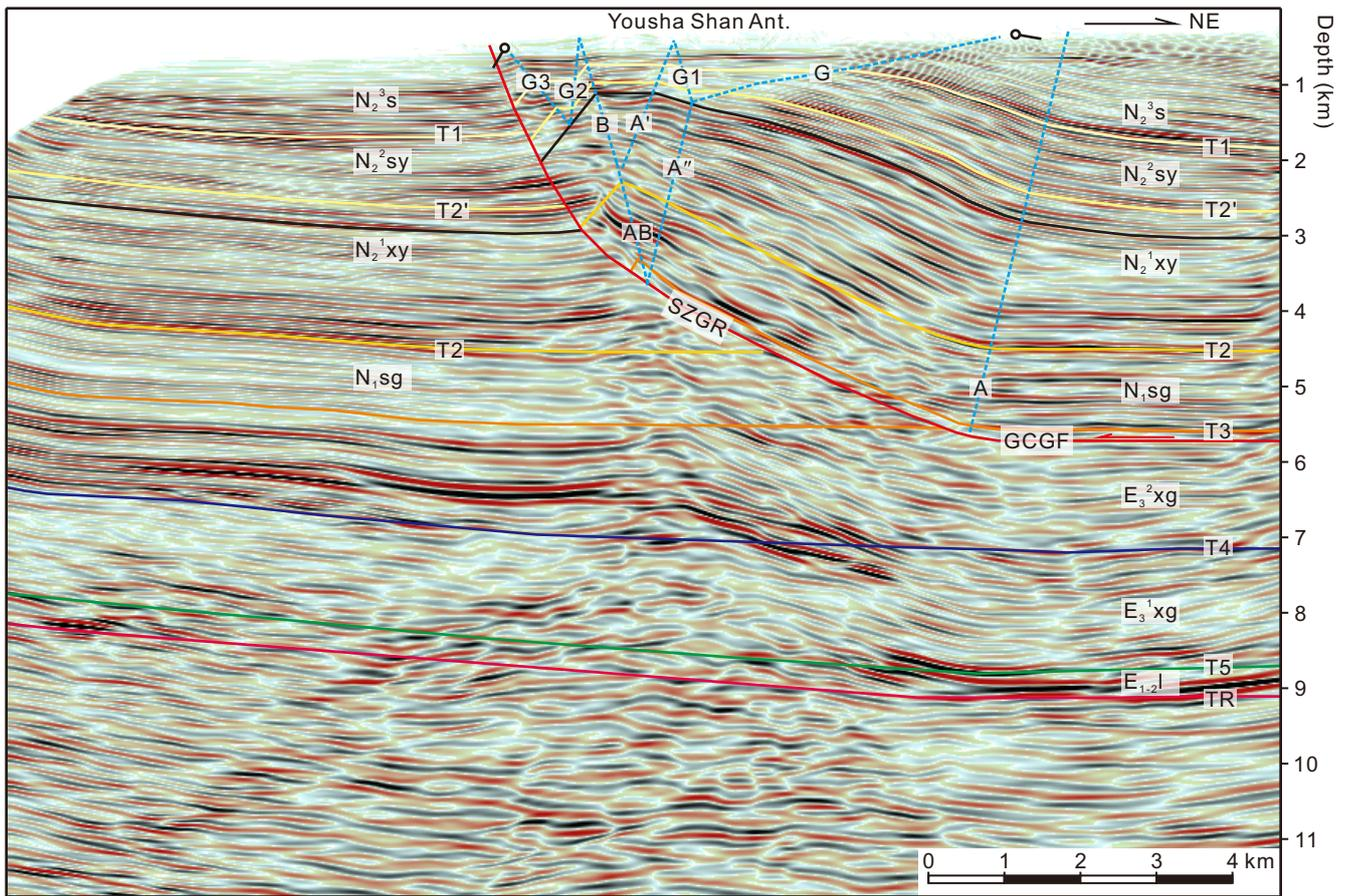
Figure 7. Interpreted seismic profile crossing the eastern segment of the SZG-YSS anticline. The vertical scale is equal to the horizontal one. See Figure 1 for location.
