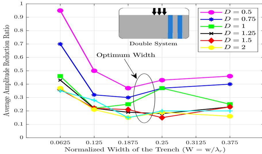
Figure 15: Influence of normalized barrier width on  $\bar{A}_r$  ( $X = 0.5$ )
