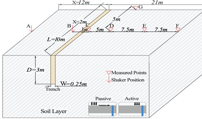
Figure 3: Measuring arrangement
