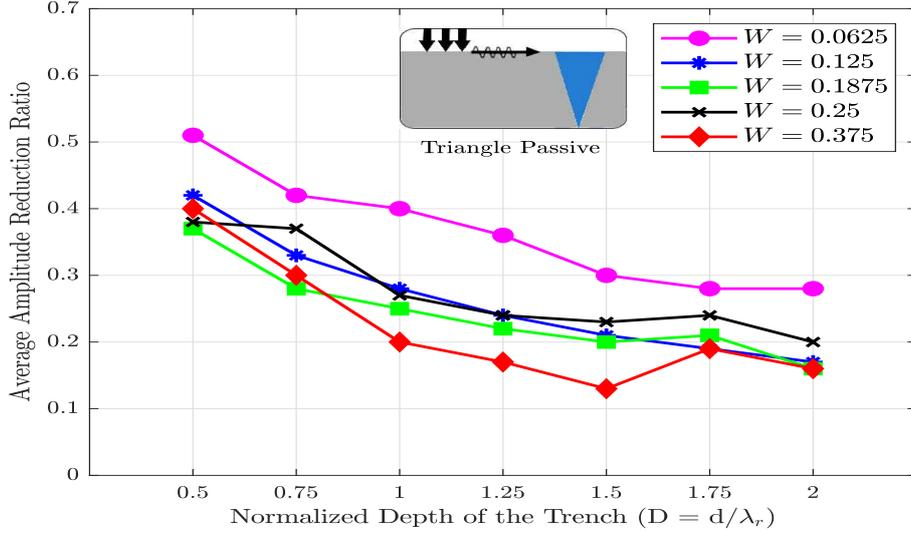
Figure 20: Influence of normalized barrier depth on  $\bar{A}_r$  ( $X = 3$ )
