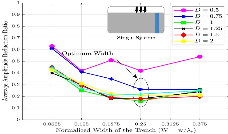
Figure 13: Influence of normalized barrier width on  $\bar{A}_r$  ( $X = 0.5$ )
