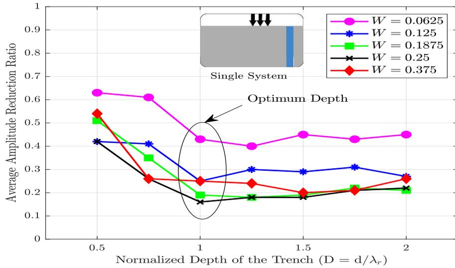
Figure 12: Influence of normalized barrier depth on  $\bar{A}_r$  ( $X = 0.5$ )
