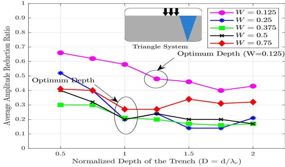
Figure 16: Influence of normalized barrier depth on  $\bar{A}_r$  ( $X = 0.5$ )
