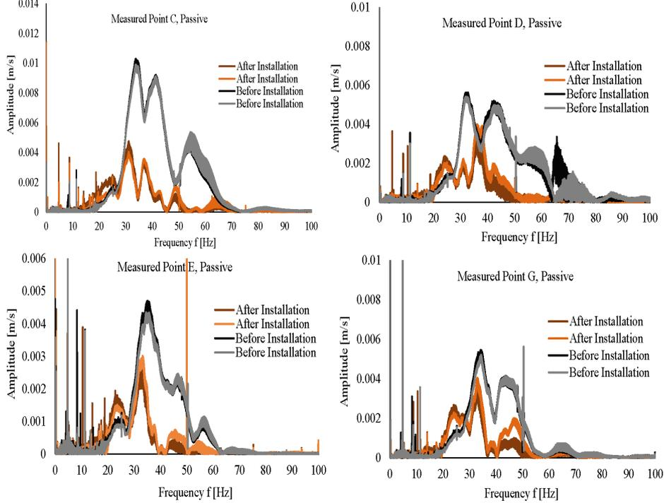
Figure 6: Representation in the frequency domain: Measuring points C, D, E, G (Passive Isolation)
