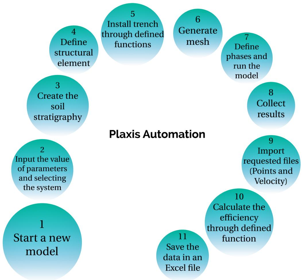
Figure 8: Automation process of Plaxis model with Python
