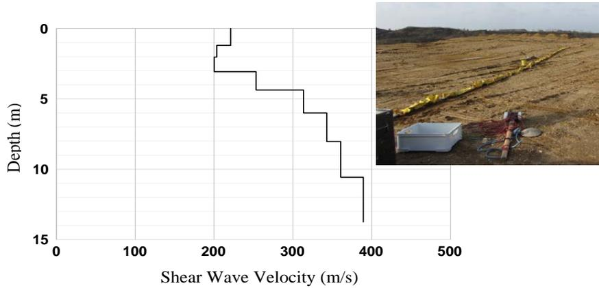
Figure 1: Shear wave velocity profile of the site
