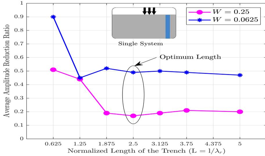
Figure 11: Influence of normalized barrier length on  $\bar{A}_r$  ( $X = 1.25$ ,  $D = 1.25$ )
