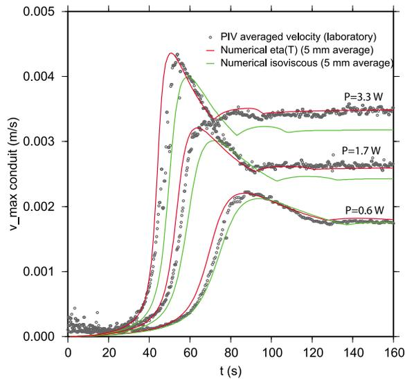
**Figure 7.** Comparison of conduit velocity (with a 5 mm by 3 mm averaging window) using the numerical simulation for various powers and the measured rheology (solid red lines, same as in Figure 6b) and those for a strictly isoviscous rheology (solid green lines).
