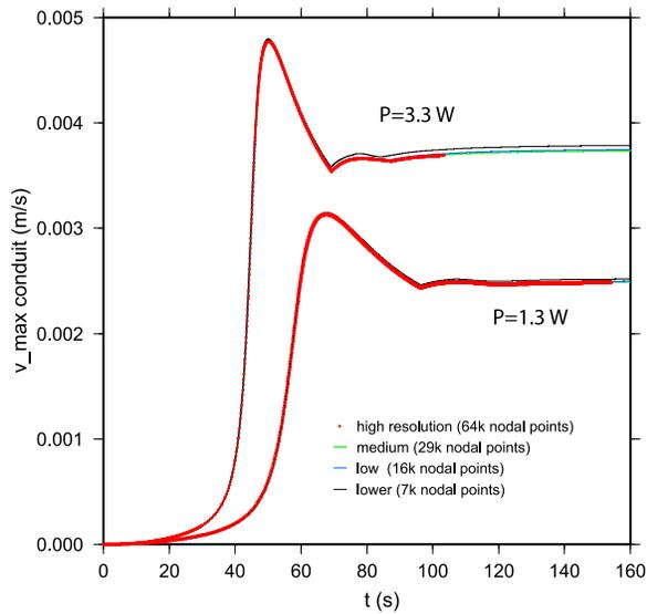
**Figure 5.** Resolution test for the numerical simulations for fluid 47V500 and powers  $P = 1.3$  and  $3.3$  W. The red dots show the results on the high-resolution mesh (with 63,683 nodal points) that was used for the numerical simulations shown in Figures 5 and 6. The green and blue curves show the results for intermediate and low resolution. The results only deviate noticeably for the higher-power model when ten times fewer nodal points are used (black curve).
