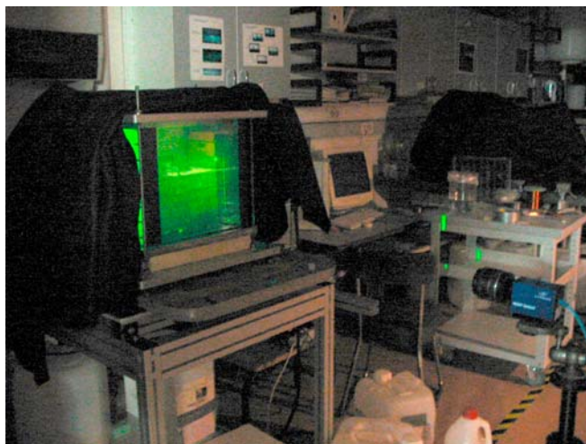
Figure 1. (a) Photo of the laboratory setup (at IPGP) demonstrating the laser sheet (in green), heater assemblage (minor bright point at base of tank), and digital camera. (b) Illustration of the tank geometry and (c) the axisymmetric finite element model. The green area in Figure 1b shows a typical photograph of a plume with temperature contours illuminated by the TLC, and the quadratic elements of the finite element mesh which has a resolution of 0.2 mm near the heater are shown in Figure 1c.
