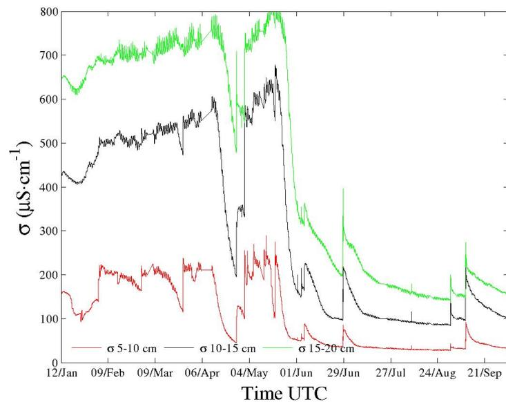
**Figure 3.** Time series over nine months of a three-channel sensor located in a remote catchment of the French Southern Alps—one point every 10 min. Minor interruptions due to power supply. Soil conductivity profile in  $\mu\text{S}\cdot\text{cm}^{-1}$ .
