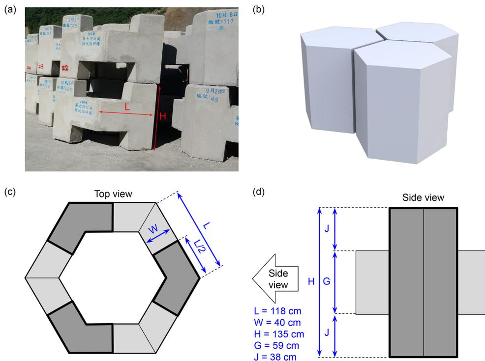
**Figure B1.** (a) Photograph of the dolosse. (b) 3-D hexagonal shape of the plain dolos as seen by the photogrammetry. (c) Top view of the actual dolos. The dark gray parts are the pillars actually touching the ground and the light gray parts are the “arms” of the dolos. (d) Side view of one dolos element. One dolos consists of three of these parts joined by the arms.
