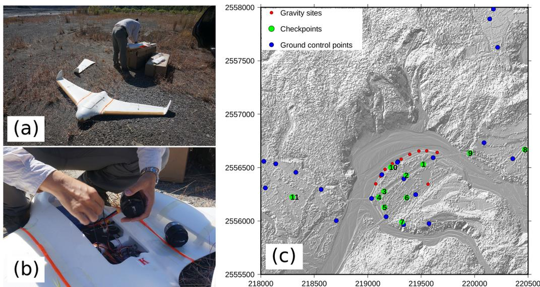
**Figure 6.** (a) Modified Skywalker X8 UAV. (b) Close-up on the central compartment of the UAV, where the camera and lens are mounted. (c) Map of the ground control points and checkpoints (numbered according to Table 4) with the shaded topography in the background. The gravity sites are also shown for reference.
