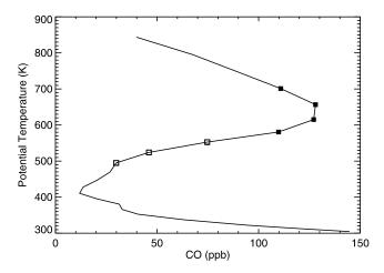
**Figure 6.** CO mixing ratio plotted against potential temperature on 20 March 2003 inside the vortex measured by MIPAS-B. Solid squares (corresponding to 24–27 km) indicate measurements identified as being under mesospheric influence owing to the elevated CO mixing ratio. Open squares (corresponding to 21–23 km) indicate the measurements considered as mesospheric in an earlier publication [*Engel et al.*, 2006].
