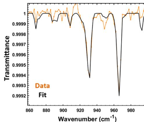
**Figure 3.** IR spectra of ammonia detected in the experiment (N<sub>2</sub>-H<sub>2</sub> 3% - 0.53 mbar – 8.4 W) and fitted to deduce ammonia density. Spectra integrated over 1h45 at 4 cm<sup>-1</sup> resolution.
