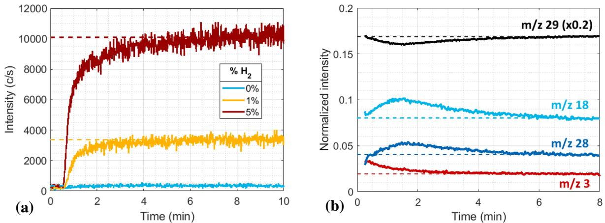
**Figure A3-1.** MS continuous acquisition in RGA and ion modes at the ignition of the plasma. (a) Intensity of  $m/z$  17 (representative of  $\text{NH}_3$  amount) at the ignition of  $\text{N}_2$  and  $\text{N}_2\text{-H}_2$  plasmas (0.53 mbar – 6.5 W). (b) Evolution of  $m/z$  3 ( $\text{H}_3^+$ ), 18 ( $\text{NH}_4^+$ ), 28 ( $\text{N}_2^+$ ) and 29 ( $\text{N}_2\text{H}^+$ ) in time until stabilization (5%  $\text{H}_2$  – 0.86 mbar – 10.5 W).
