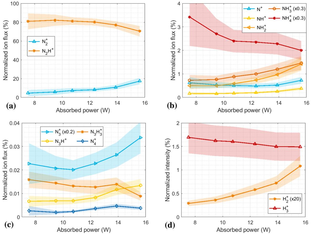
**Figure 13.** Normalized positive ion fluxes (a,b,c) or intensities (d) as function of the power absorbed by the plasma. Conditions with 5%  $H_2$  and 0.9 mbar (55 sccm).
