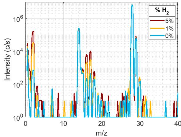
**Figure 4.** MS spectra during plasma (0.91 mbar,  $\sim 11$  W) in  $\text{N}_2$  and  $\text{N}_2$ - $\text{H}_2$  at different percentages of  $\text{H}_2$ .  $\text{N}_2$  has fragments at  $m/z$  7, 14, 15, 28, 29, 30.  $\text{H}_2$  is visible at  $m/z$  2.  $m/z$  16 and 17 are mainly associated to ammonia. Traces of water are detected at  $m/z$  18. The lower detection limit is at  $\sim 30$  c/s.
