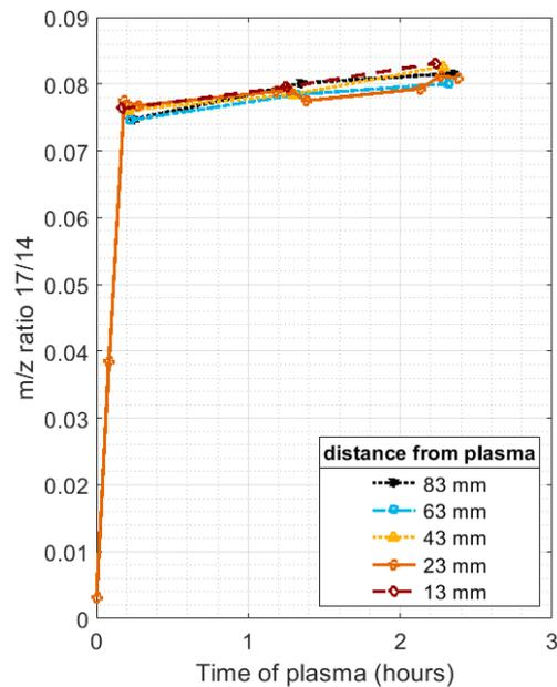
**Figure A2-1.** Variation of m/z ratio 17/14 (representative of ammonia) in time and distance from plasma (0.53 mbar – 3% H<sub>2</sub> – 8.4 W).
