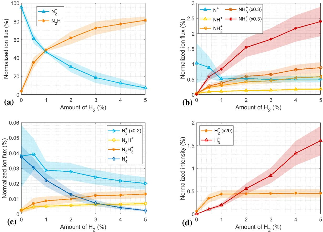
**Figure 11.** Normalized positive ion fluxes (a,b,c) or intensities (d) as function of the percentage of  $H_2$  injected in the experiment. Conditions with 0.9 mbar (55 sccm) and  $\sim 10$  W absorbed power (405 V<sub>RF,pp</sub>).
