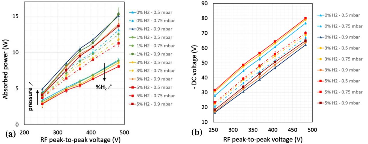
**Figure 8.** (a) RF power absorbed by the plasma and (b) self-bias potential  $V_{DC}$  as function of  $V_{RF,pp}$  in all the conditions studied here (various  $V_{RF,pp}$ , % of H<sub>2</sub> and pressure).
