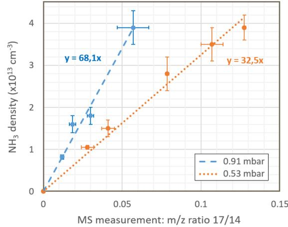
**Figure A2-2.** Calibration of MS measurements of  $\text{NH}_3$  with IR data. Experiments done at 2 different pressures (0.91 and 0.53 mbar) in a  $\text{N}_2\text{-H}_2$  plasma discharge, for a same RF peak-to-peak voltage of 480 V (at resp. 14 and 8.5 W).
