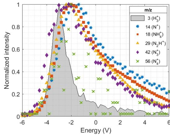
**Figure A4-2.** Energy scans for different ions in a  $N_2$ - $H_2$  plasma at 0.80 mbar. The extractor was fixed to -40 V. Note: the reference of energy axis is not calibrated and is certainly shifted of a few volts.
