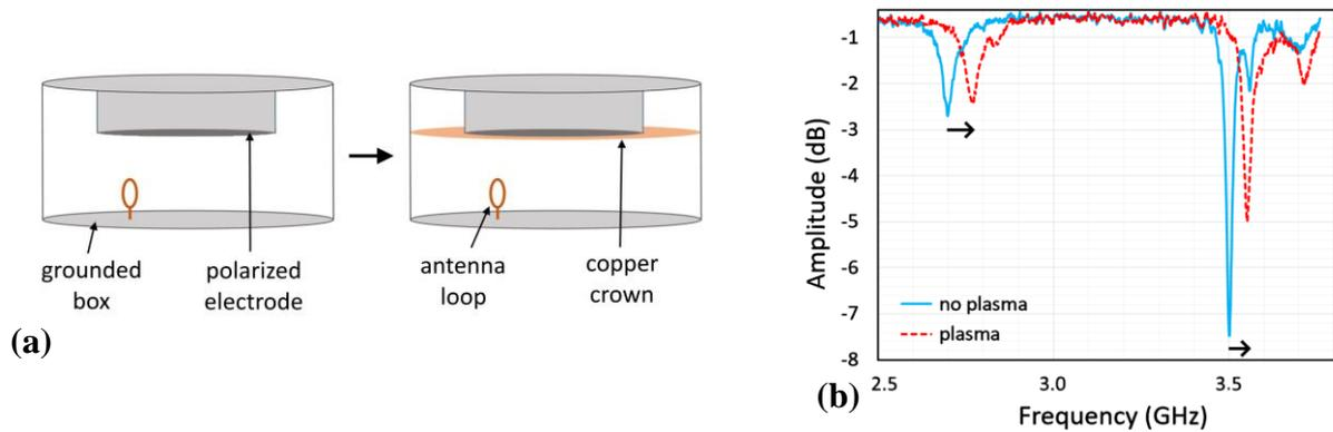
**Figure 2.** Electron density measurement. (a) Scheme of the installation of a copper crown between the polarized electrode and the confining grounded box to improve the signal. (b) Spectra showing the resonant frequencies in the box, before and after plasma ignition (0.91 mbar –  $N_2$ - $H_2$  5% - 13.5 W)
