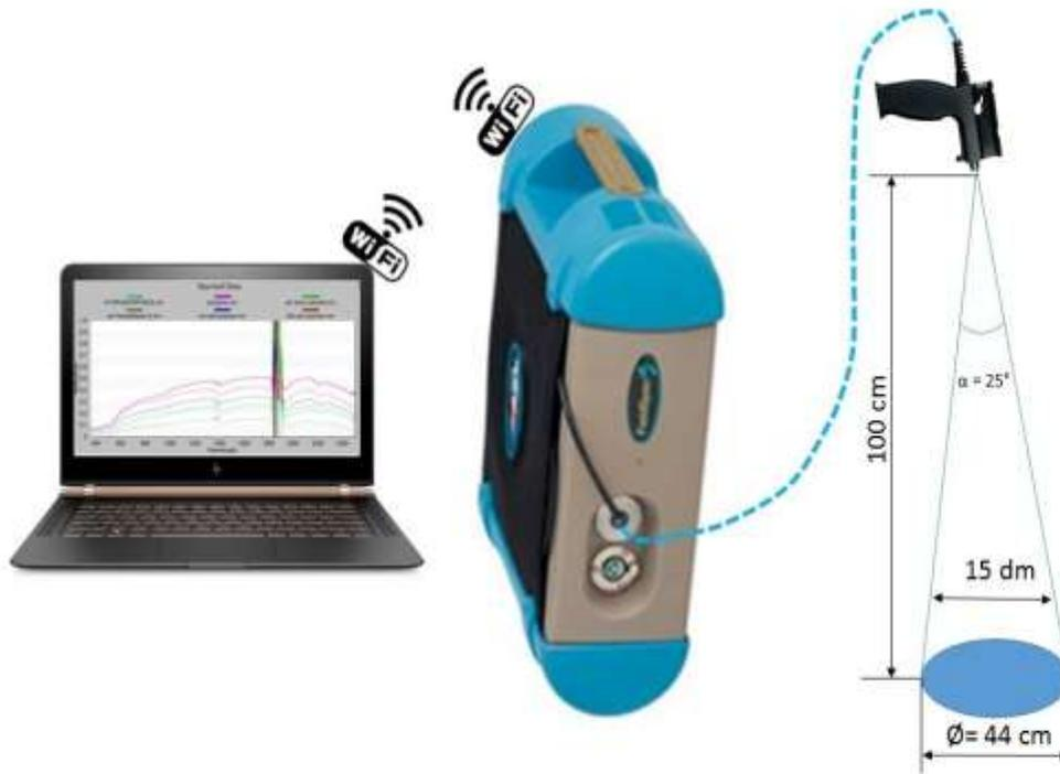
Figure 2: Schema illustrating the principle of soil reflectance acquisition using the spectroradiometer ASD Fieldspec III Pro.
