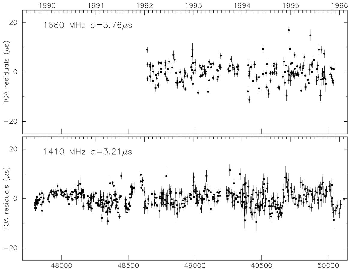
**Fig. 2.** TOA residuals of the timing data obtained on the millisecond pulsar PSR B1821-24 at the Nançay radiotelescope. (bottom) Residuals from timing observations at 1410 MHz characterized by a post-fit rms of  $3.21\mu\text{s}$ . (top) Residuals from 1680 MHz data characterized by a rms of  $3.76\mu\text{s}$ . Parameters solved are  $P, \dot{P}, \ddot{P}, P^{(3)}, \alpha, \delta, \mu_\alpha$  and  $\mu_\delta$ .
