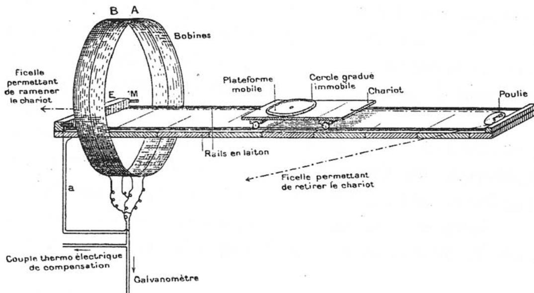
**Figure 11.** Mobile tray and coils used in conjunction with a ballistic galvanometer by *Chevallier* [1925b] to measure rock sample magnetization. Reprinted from *Chevallier* [1925b, Figure 4] with kind permission from Springer Science and Business Media.
