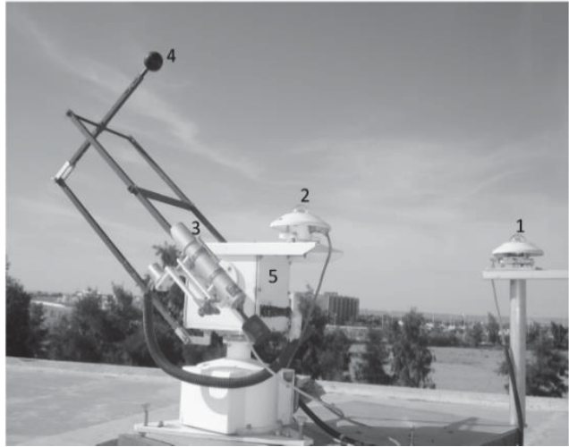
Figure 6. Radiometric station for measuring global, direct and diffuse solar radiation: (1) Pyranometer for measuring the global solar irradiance. (2) Pyranometer for measuring the diffuse. (3) Pyrliometer for measuring the direct solar irradiance, (4) Shaded pyranometer. (5) The 2-axis solar tracker.
