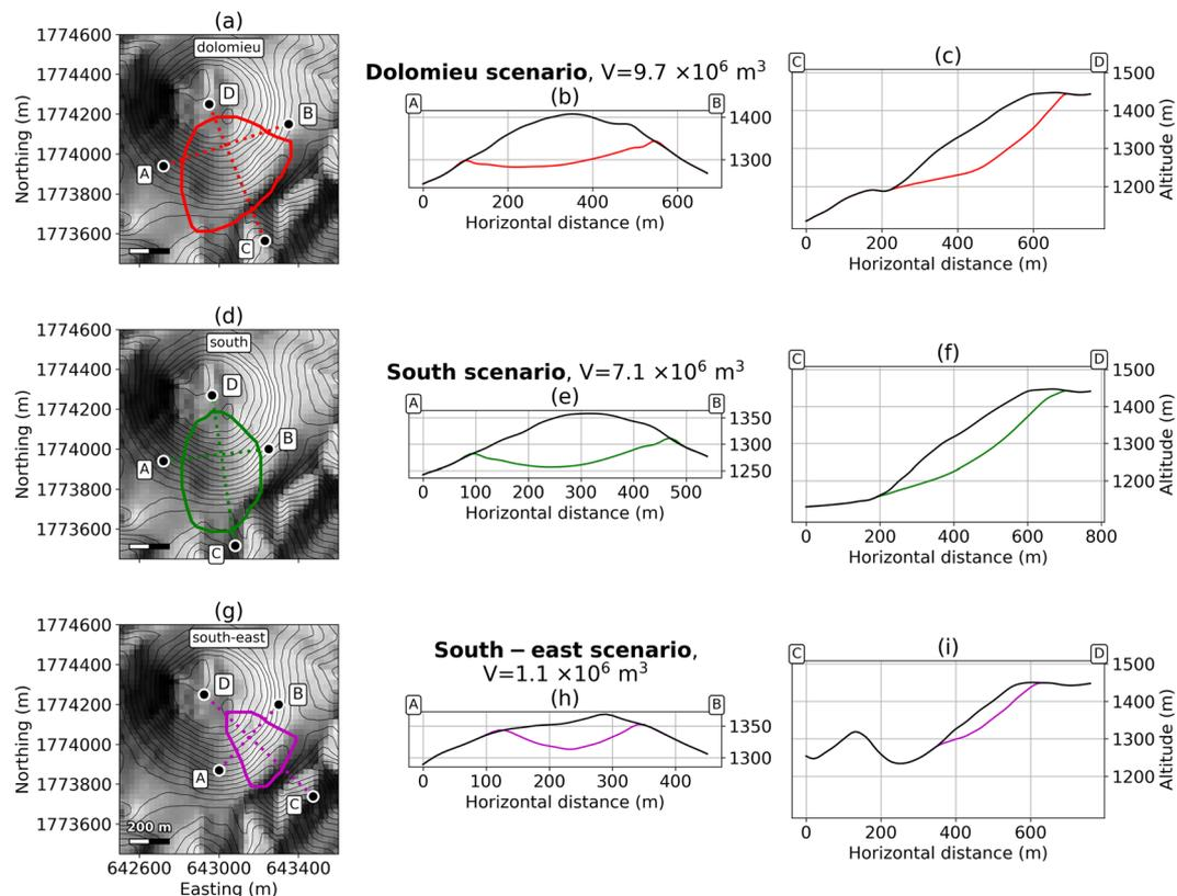
**Figure 4.** Collapse geometries of superficial scenarios. (a,d and g) respectively display the extent of *dolomieu*, *south* and *south-east* scars. (b,c,e,f,h,i) are cross-sections of the initial (black line) and post-collapse (colored line) topographies, respectively for *dolomieu*, *south* and *south-east* scenarios. Cross-sections extents are indicated by the letters A, B, C, D. The DEM is from IGN BDTopo, coordinates: WGS84, UTM20N. The contour interval is 20 m.
