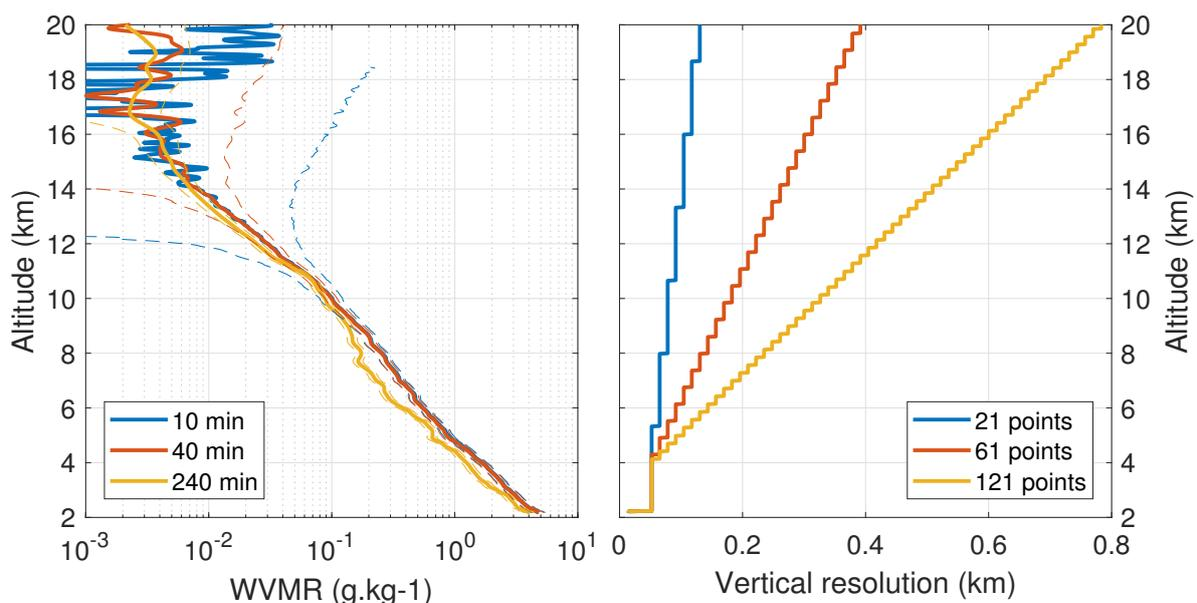
**Figure 4.** Mean profiles integrated over 10 min (solid blue line), 40 min (solid orange line) and 240 min (solid yellow line) with their total uncertainty (dotted lines) (**left**), and the associated vertical resolution (**right**) according to the altitude above sea level.
