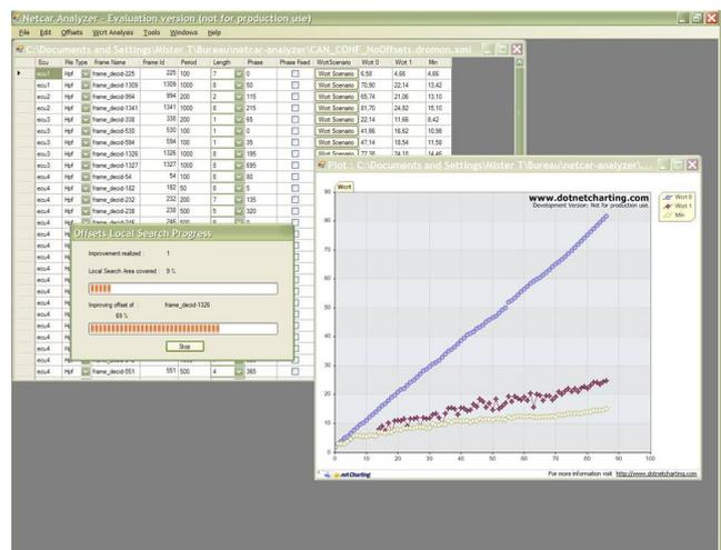
Figure 1: Screenshot of NETCAR-Analyzer during an optimization run. The right-hand graphic shows the response times (by decreasing priority) for different offset configurations. The spreadsheet in the background contains the set of frames, the different offset configurations tested, the corresponding WCRT and certain characteristics of the ECUs, such as the queuing policy at the microcontroller level (e.g., FIFO or prioritized).
