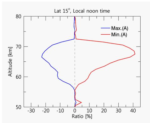
Figure 2: Estimated solar heating rate variations during the past decade at low latitudes ( $15^\circ$ ) compared to the mean albedo condition. This calculation assumes that the abundance variations of the unknown absorber in the cloud top level is responsible on the observed 365-nm albedo changes.
