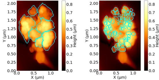
Figure 1: MIDAS topographic image of dust stuck to an AFM tip with its major units (left) and surface structure/sub-units (right)
