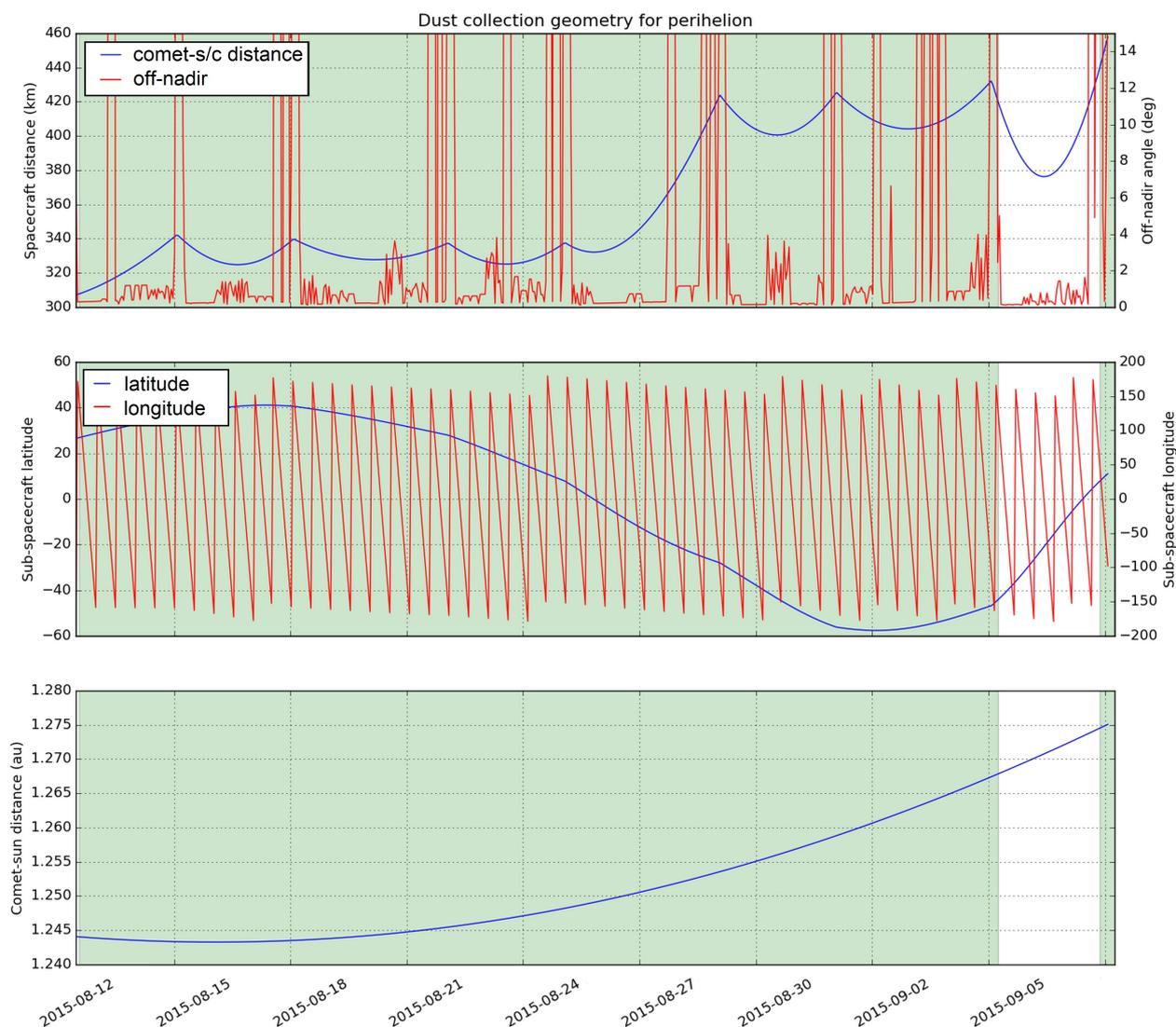
**Fig. A.1.** Collection geometry for particle G (see Figs. 1 and 2). Green shaded regions show the periods when particles could be collected. *Upper panel:* comet-spacecraft distance and off-nadir pointing, *middle panel:* latitude and longitude, and *bottom panel:* comet-Sun distance.
