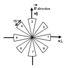
**Figure 2.** Angular coverage of the electron instrument on Helios 1: eight angular sectors  $\theta_i$ , with widths  $\delta\theta_i = 15^{\circ}$ , are spaced  $45^{\circ}$  apart from one another. This coverage is used to compute the "average electron velocity distribution functions" (see the text for more details).
