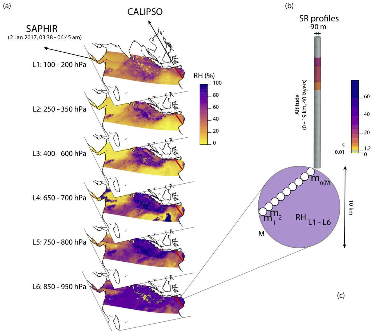
**Figure 1.** (a): RH (mean) observed by SAPHIR for all six pressure layers in the Indian Ocean on 2 January 2017 between 03:38 and 06:45 UTC. Overlaid is the CALIPSO track line (red line). (b): example of the SR profile measured by CALIPSO. (c): schematic representation of SAPHIR–CALIPSO co-location:  $M = 1, \dots, N$  SAPHIR measurements at coarse resolution encapsulating  $m = 1, \dots, n(M)$  finely resolved CALIPSO observations.
