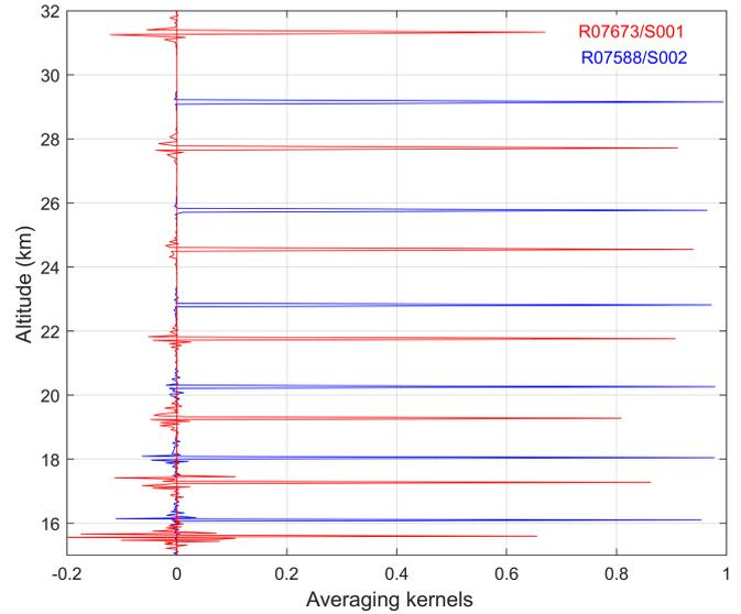
**Figure 6.** Examples of averaging kernels at selected altitudes, red: oblique occultation R07673/S001, blue: vertical occultation R07588/S002. The detailed information about these occultations can be found in the caption of Fig. 4.
