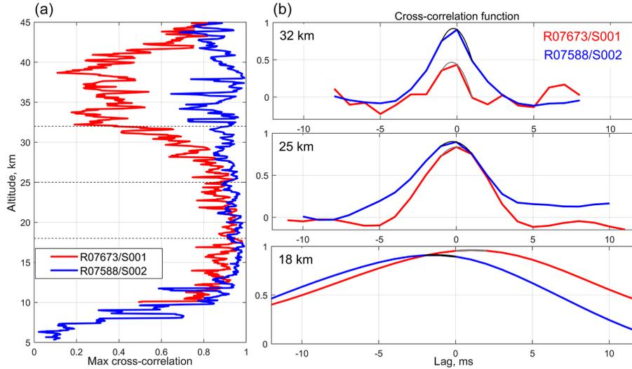
Figure 4. (a) Maximum of cross-correlation function for two GOMOS occultations: R07673/S001 (64° S 68° W,  $\beta = 23^\circ$ , 19 August 2003 04:09:23 UTC), red line, and R07588/S002 (35° S 135° W  $\beta = -2.6^\circ$  13 August 2003 07:28:35 UTC), blue line. (b) Examples of cross-correlation functions at selected altitudes and their fit with the parabola (black and grey lines).
