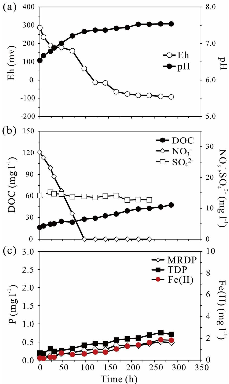
Figure 6. Dynamics of parameters during anaerobic incubation of sediment S. (a): Eh and pH; (b): dissolved organic carbon (DOC), NO<sub>3</sub><sup>-</sup> and SO<sub>4</sub><sup>2-</sup> concentrations; (c): molybdate-reactive dissolved P (MRDP), total dissolved P (TDP) and Fe(II) concentrations.
