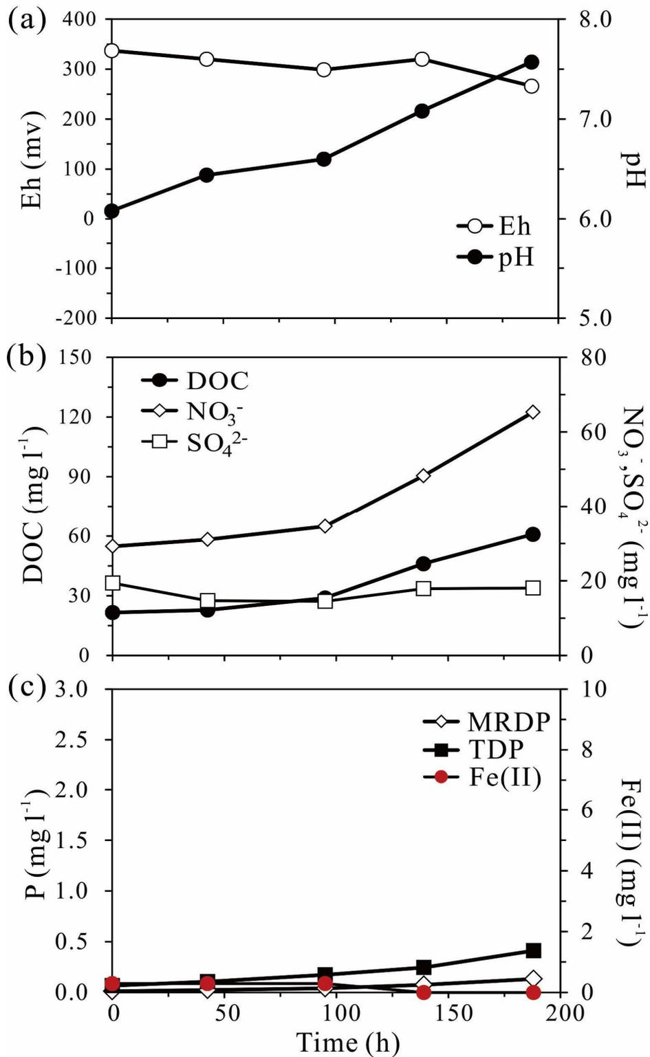
Figure 5. Dynamics of parameters during aerobic incubation of soil B. (a): Eh and pH; (b): dissolved organic carbon (DOC), NO<sub>3</sub><sup>-</sup> and SO<sub>4</sub><sup>2-</sup> concentrations; (c): molybdate-reactive dissolved P (MRDP), total dissolved P (TDP) and Fe(II) concentrations.
