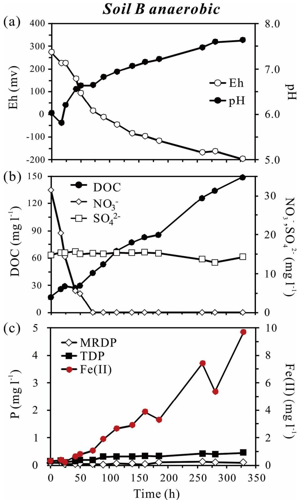
Figure 2. Dynamics of parameters during anaerobic incubation of soil B. (a): Eh and pH; (b): dissolved organic carbon (DOC), NO<sub>3</sub><sup>-</sup> and SO<sub>4</sub><sup>2-</sup> concentrations; (c): molybdate-reactive dissolved P (MRDP), total dissolved P (TDP) and Fe(II) concentrations.
